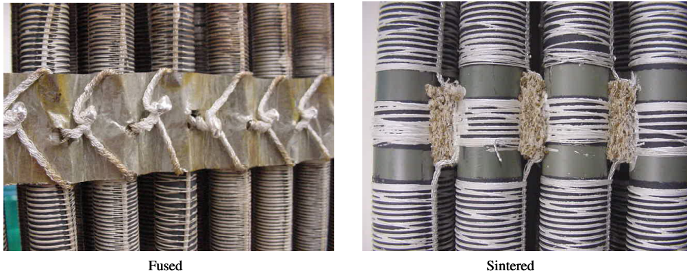
Figure 9 Fused and Sintered Current Collection Methods
