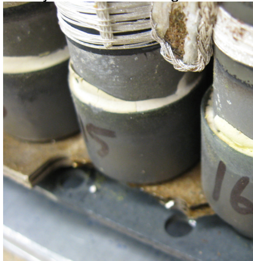
Figure 43 Cemented Joint after 9000 hrs
