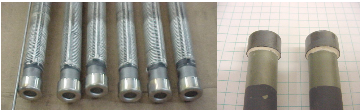
Figure 8 Cells with Brazed Caps and Cells with Cemented Caps
