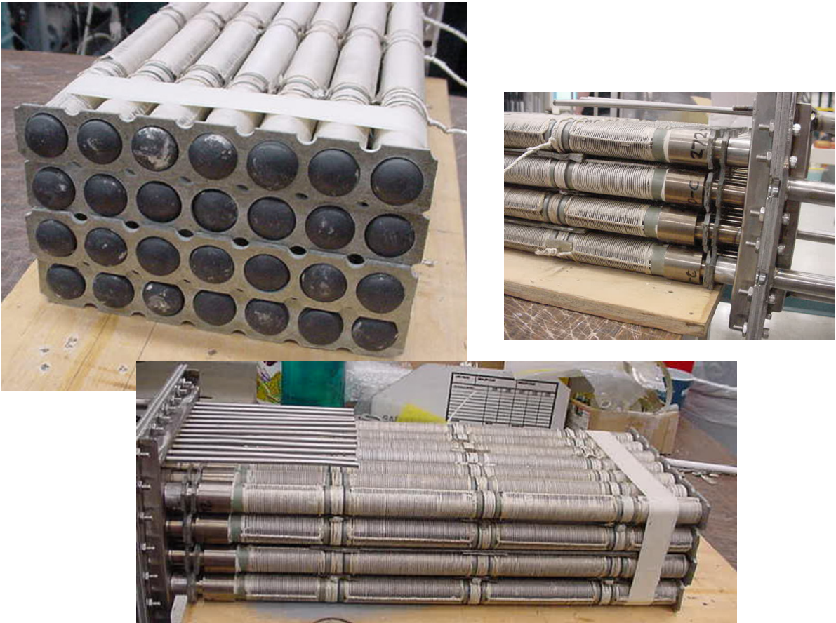
Figure 10 Sintered Bundle with 22 mm Diameter Cells
