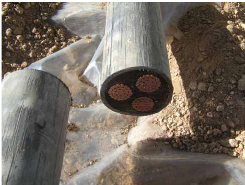
Photograph 22: Cross Section of Lead-Sheathed Cable, 02/06/2013
