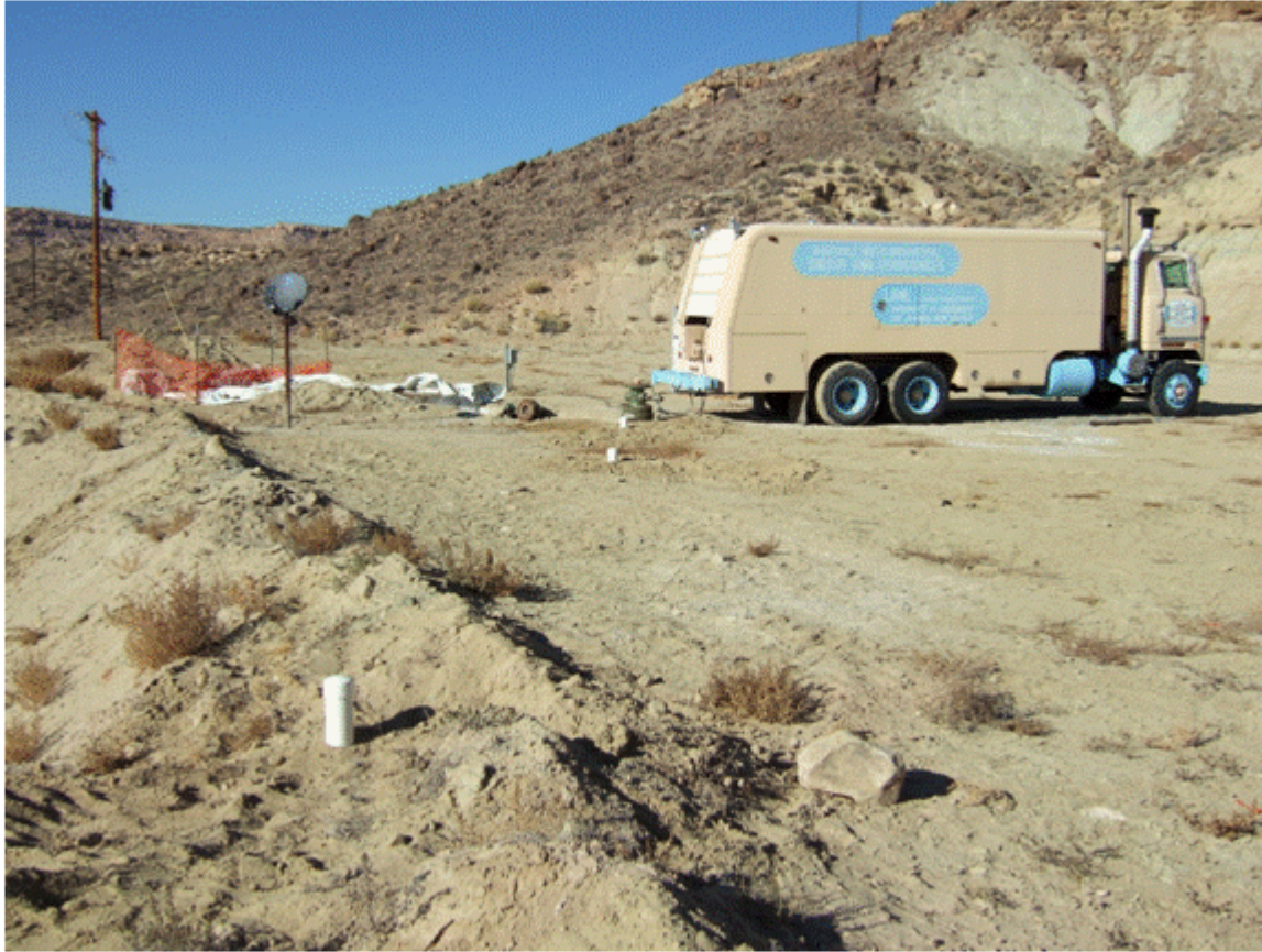
Figure 16. Photo showing three white-color caps of one-meter holes for electrodes “C313SEn”, “C313SEm” and “C313SEf” installed near the C313SE wellhead. An Ag-AgCl electrode itself is set on the bottom of the each hole.
