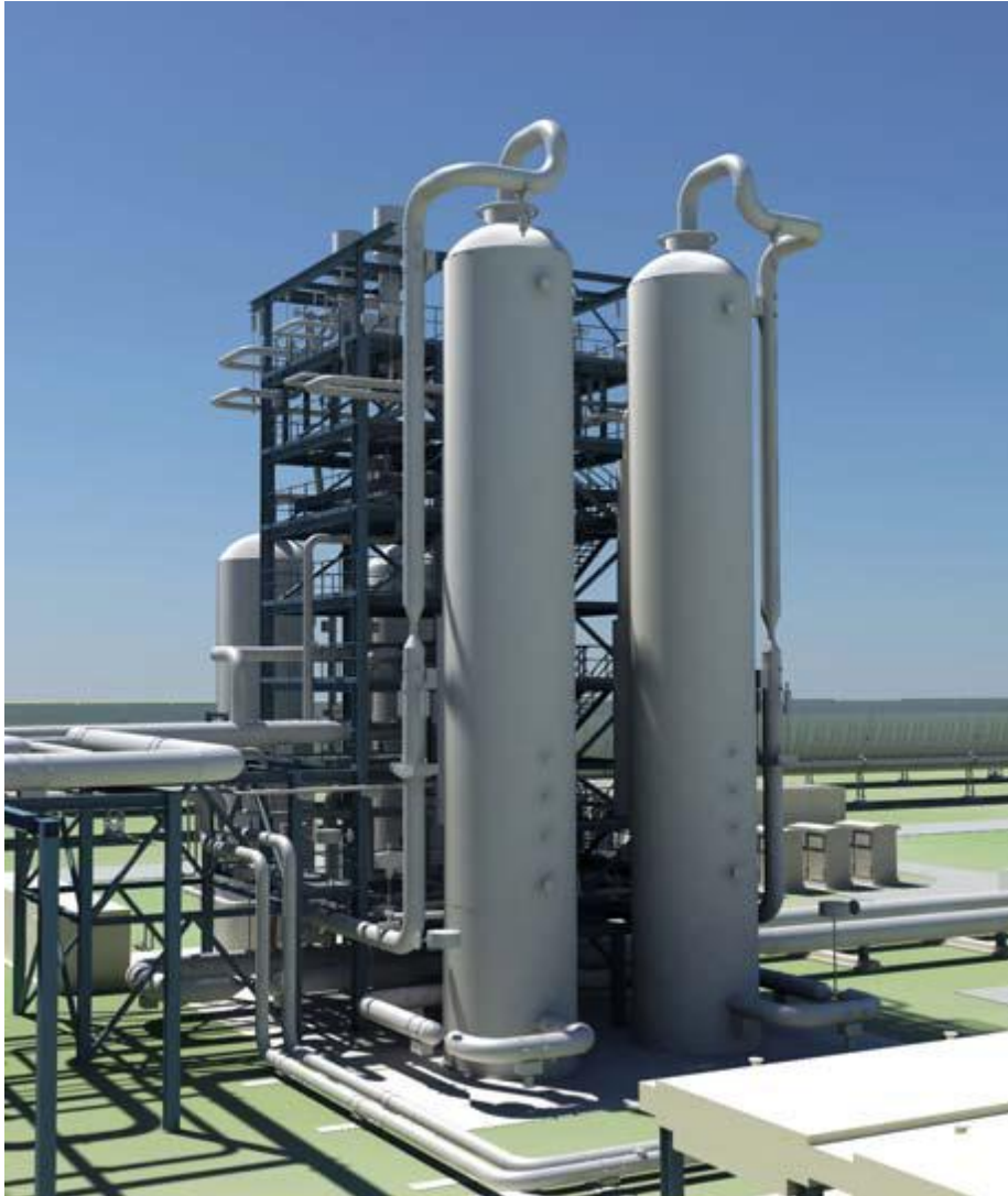
Figure 4. 3D model view of once-through (BENSON® technology) boiler
