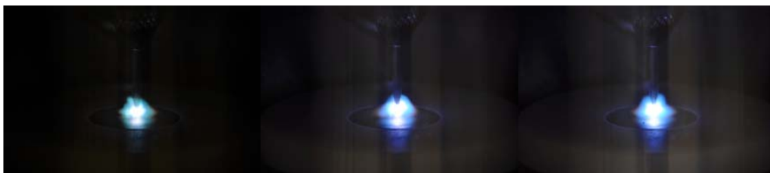
Figure 4. Effect of exposure time on image capture of spark (0.05 \mu F-5000 V) on blank sample holder, aperture f/20, for 0.5 seconds (left), 1 second (center), and 2 seconds (right).
