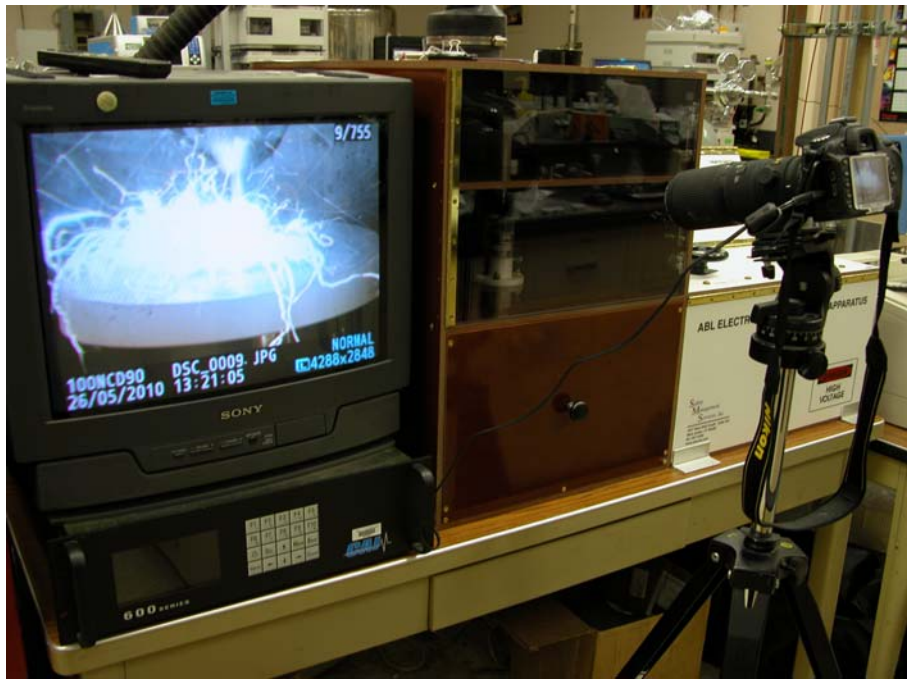
Figure 3. SLR Camera detection method for ESD testing, including the SLR camera body, 200-mm lens, tripod, and television, displaying the results of a test.
