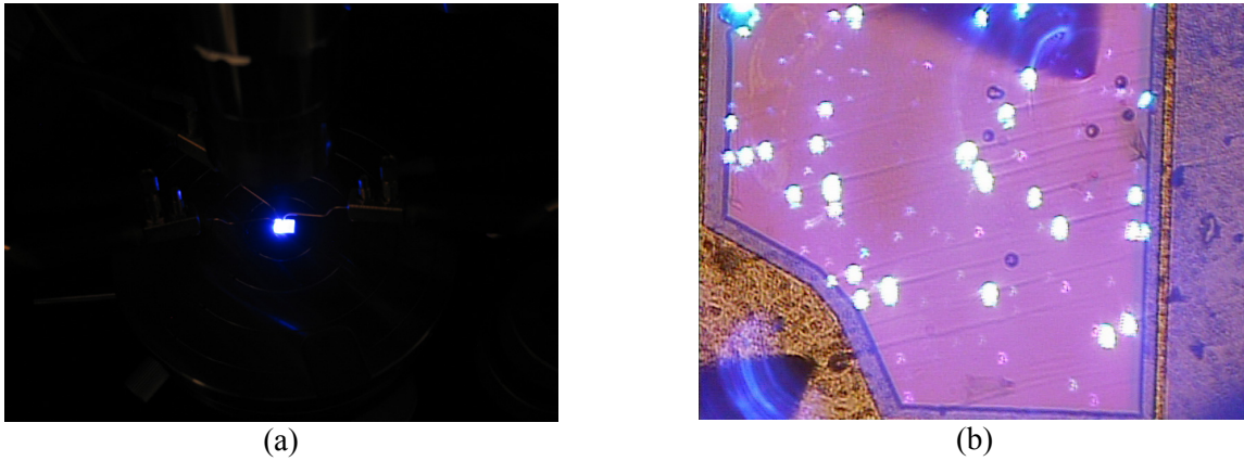
Figure 8: (a) Bird's eye view of light emission and (b) picture of light output (at low current level) from fabricated LED devices grown on a (11-20) a -plane FS-GaN substrate.
