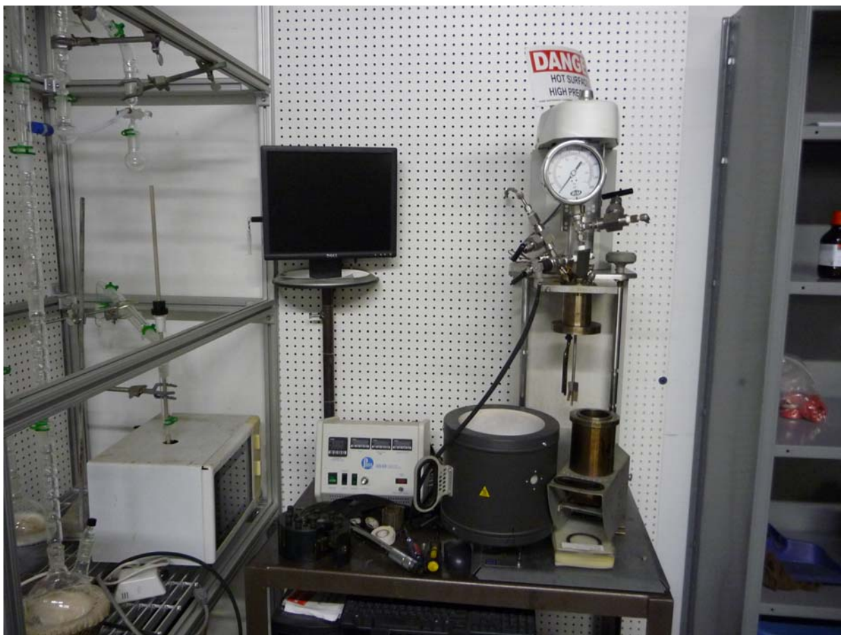
Figure 24. The bench scale stirring catalytic reactor system
