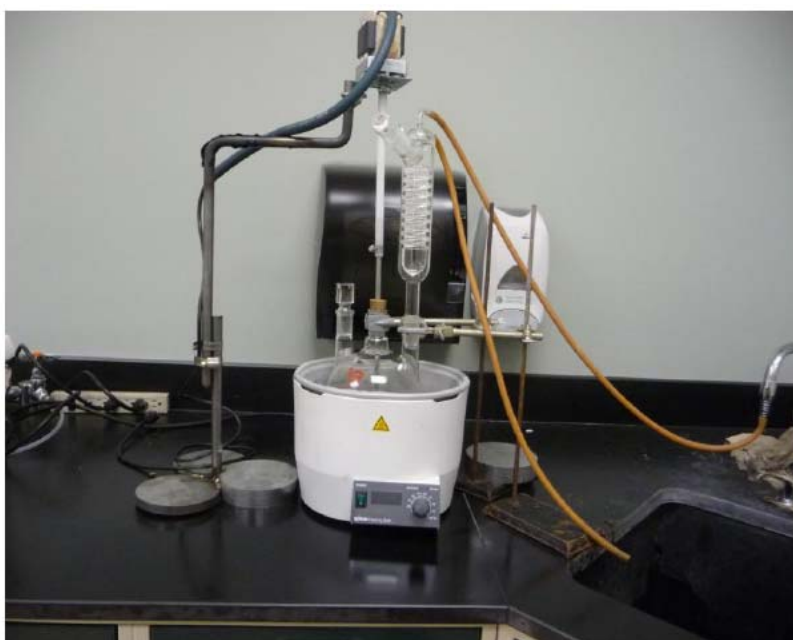
Figure 2. Picture of the ambient pressure stirring reactor
