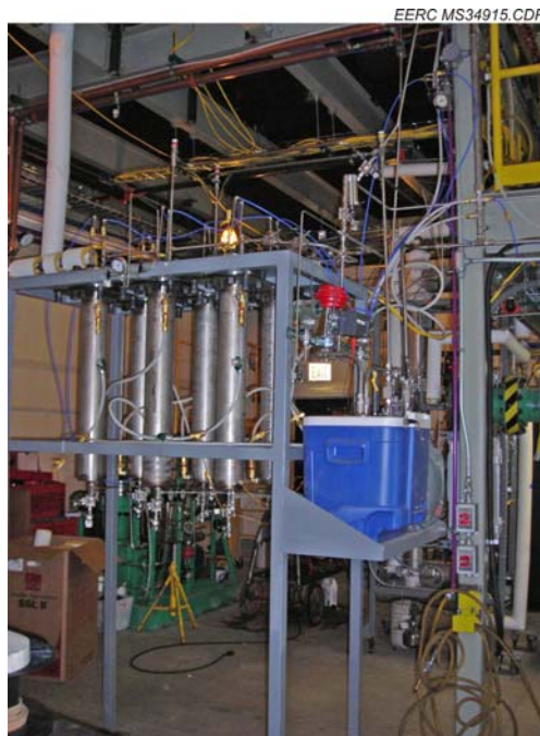
Figure 8. Photograph of the quench system for steam condensation with back-pressure control valve.
