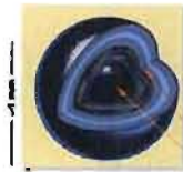
Ceramic Coatings Fuel Kernel
