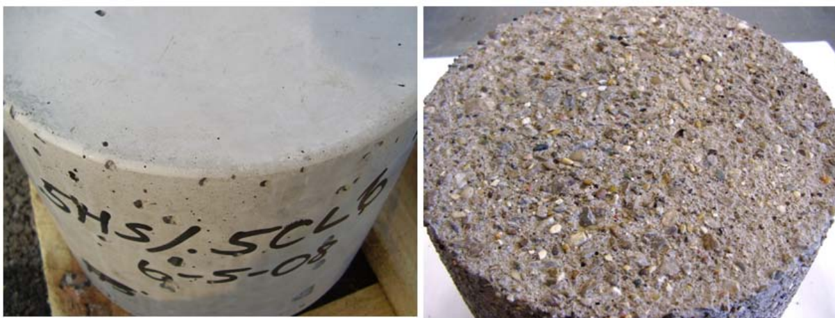
Figure 40. Specimen of clinkerless cement concrete; after 1 day exposure (left) and after 2 years exposure (right). Note the exposure of the aggregate caused by gradual dissolution of the cement component.
