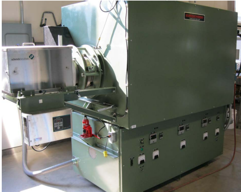
Figure 24. Finalized rotary kiln configuration (input side) with upgraded wiring and cement, raw material, feeder system.
