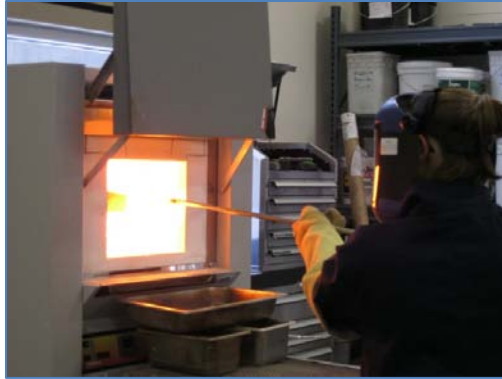
Figure 9. Box furnace used to produce batch quantities of cement for testing.
