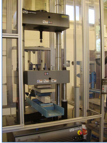
Figure 10. Instron 600DX universal closed-loop testing instrument.
