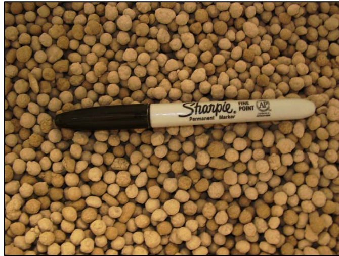
Figure 31. CSAB#4 pelletized raw materials.
