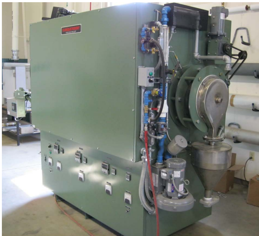
Figure 25. Finalized rotary kiln configuration (output side).
