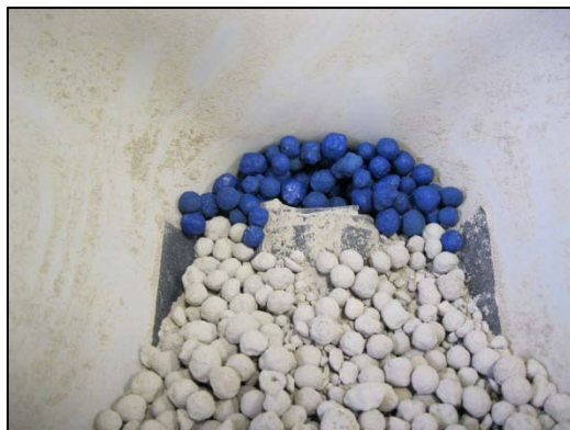
Figure 26. Blue pellets passing through material feeder into the rotary kiln during the residence-time evaluation.
