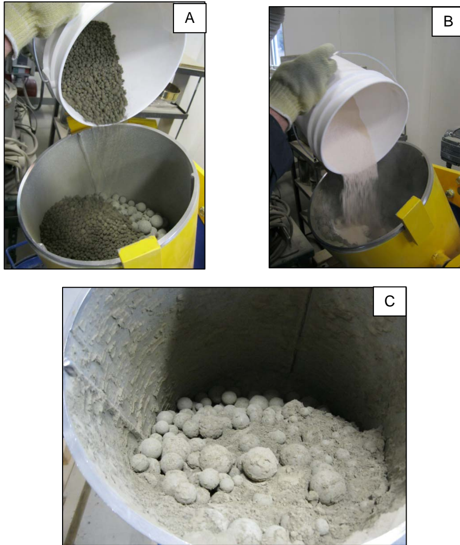
Figure 29. A) CSA Clinker product added to ball mill; B) Anhydrite added to milled CSA clinker; C) Final cement product in ball mill.
