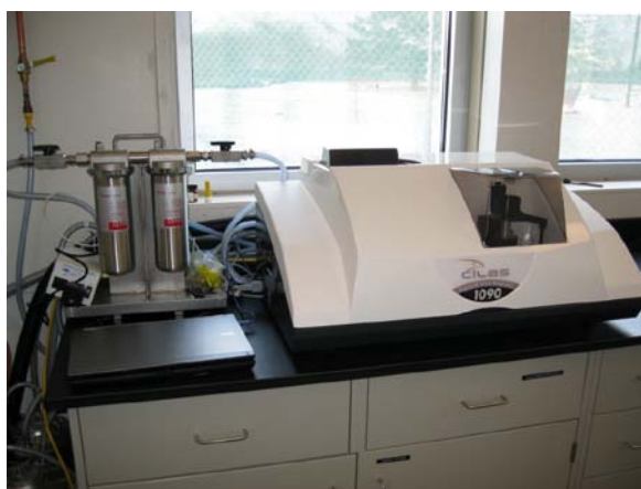
Figure 18. Cilas 1090 particle size analyzer with alcohol recirculation system (on the left).
