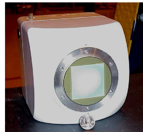
Princeton Instruments Quad-Ro CCD (Streak camera detector)
