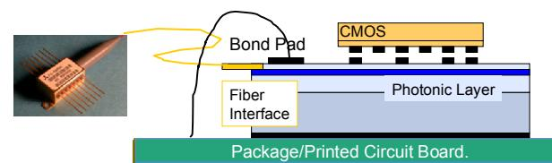
Photonic/electronic integration working towards a 100 fJ/bit link energy
