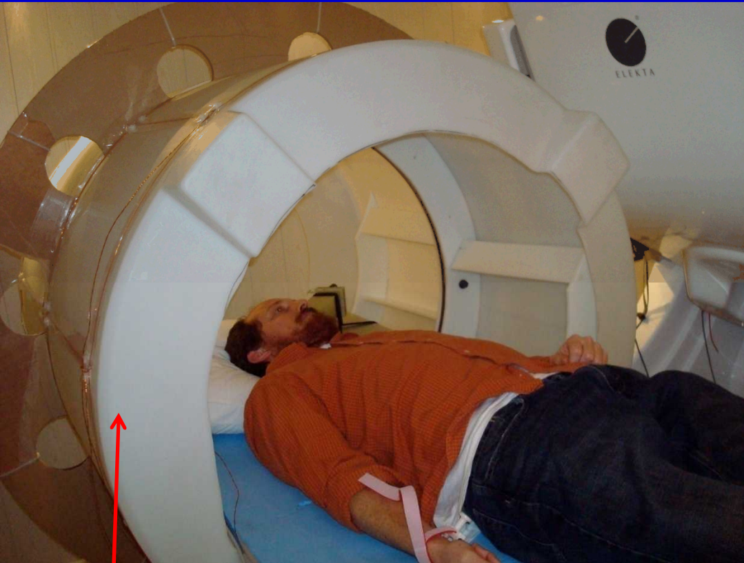
18-coil field cancellation system for reducing the field from \sim 100 nT to < 1 nT
