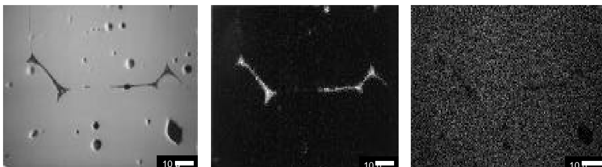
Fig. 3-6. Elemental mapping by WDS of \text{CeO}_2 + 2 \text{ wt } \% \text{Ga}_2\text{O}_3 sintered at 1650^\circ\text{C} for 6 h: (left) SEM of scanned area; (middle) distribution of gallium; (right) distribution of cerium.
