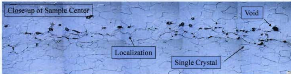
Explosively Loaded Tantalum Experiment 6 mm thick PETN Beneath Sample – Center Detonated Soft Sample Recovery
