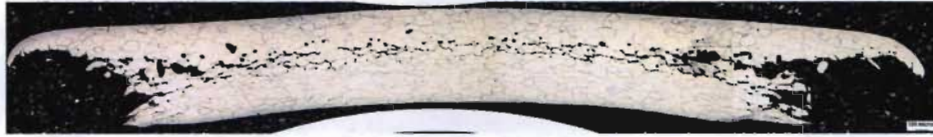
Explosively Loaded Tantalum Experiment 6 mm thick PETN Beneath Sample – Center Detonated Soft Sample Recovery
