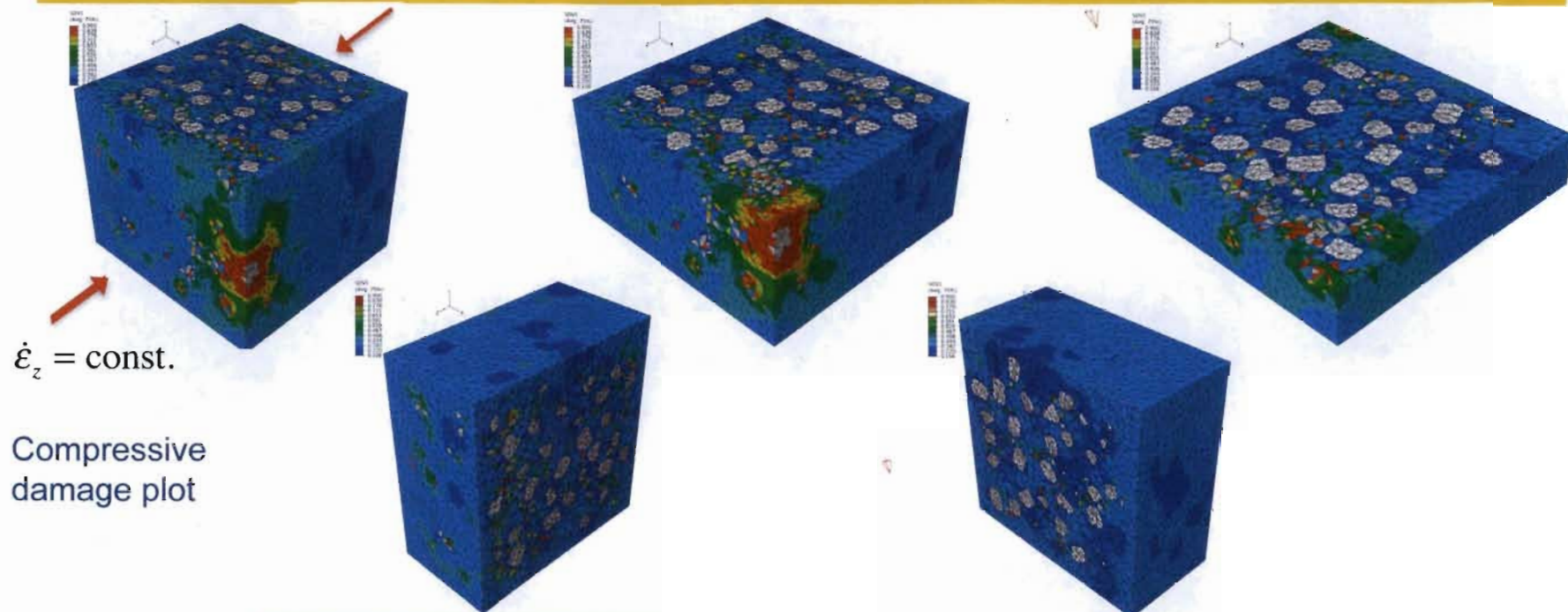
Local (element) stress-strain in the z-direction
