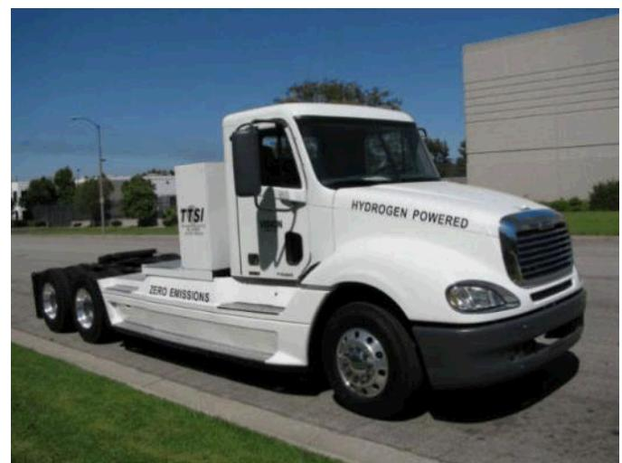
**Vision Industries C8 Fuel Cell Hybrid-Electric Drayage Truck**
