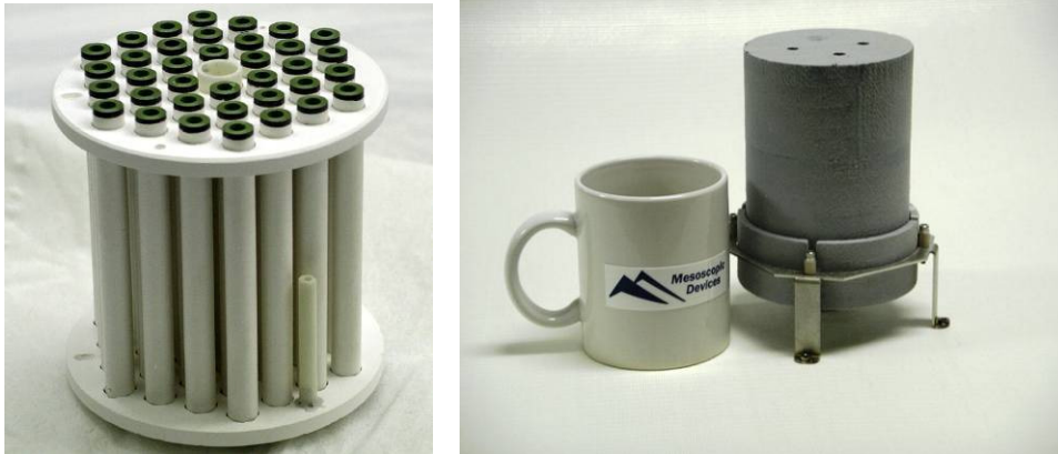
Figure 5-3. Stack and hot zone for 75 W portable generator.
