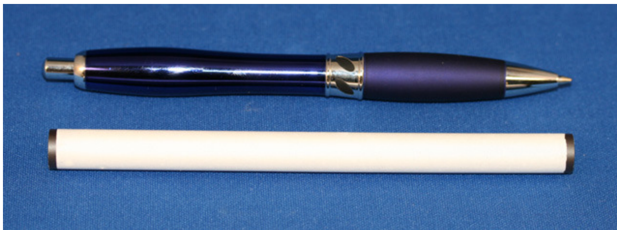
Figure 5-1. Ø10x136 mm tubular cell.
