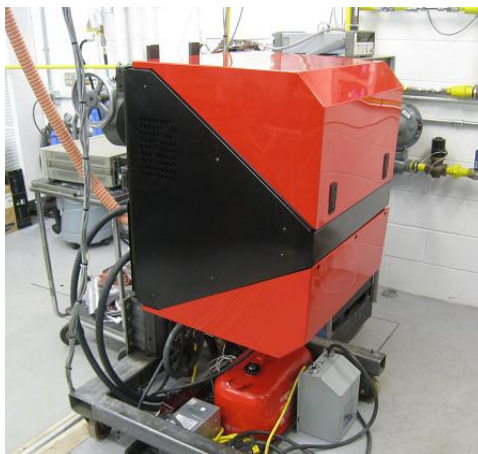
Figure 7-17: Solid model of SOFC APU assembly and associated hardware
