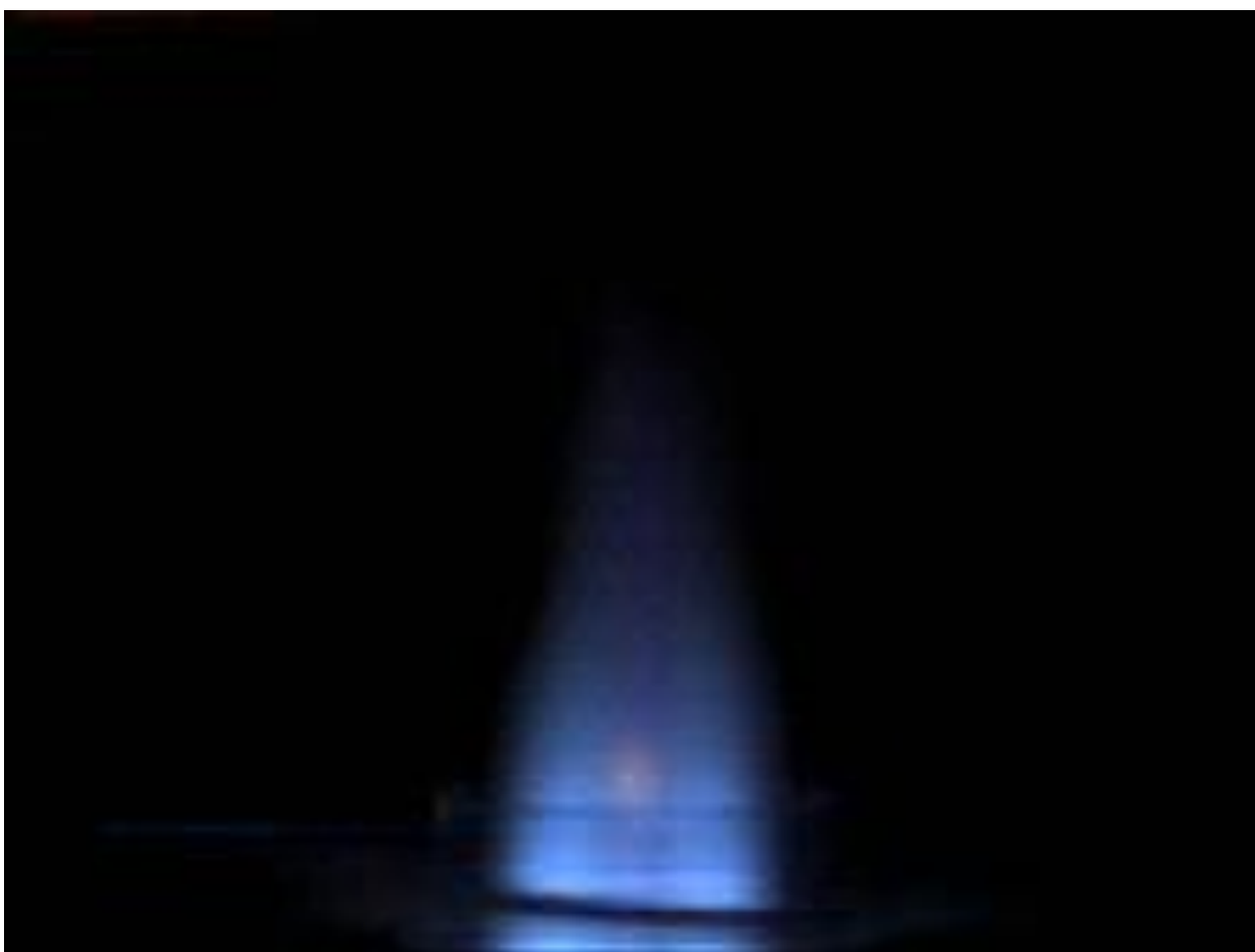
Figure 8b. Single image of a particle cloud during the ablation of NIST 610 glass. The brightest emission surrounding the particle is off-center from the larger cloud, signifying the cloud has drifted since it vaporized from the particle.
