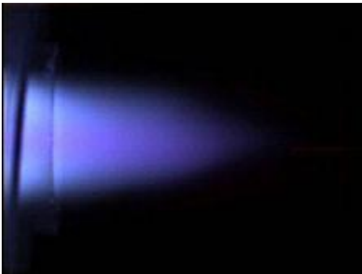
Figure 6. High speed image of the ICP during the introduction of femtosecond laser ablation generated aerosol of NIST 610 glass with helium sample gas.
