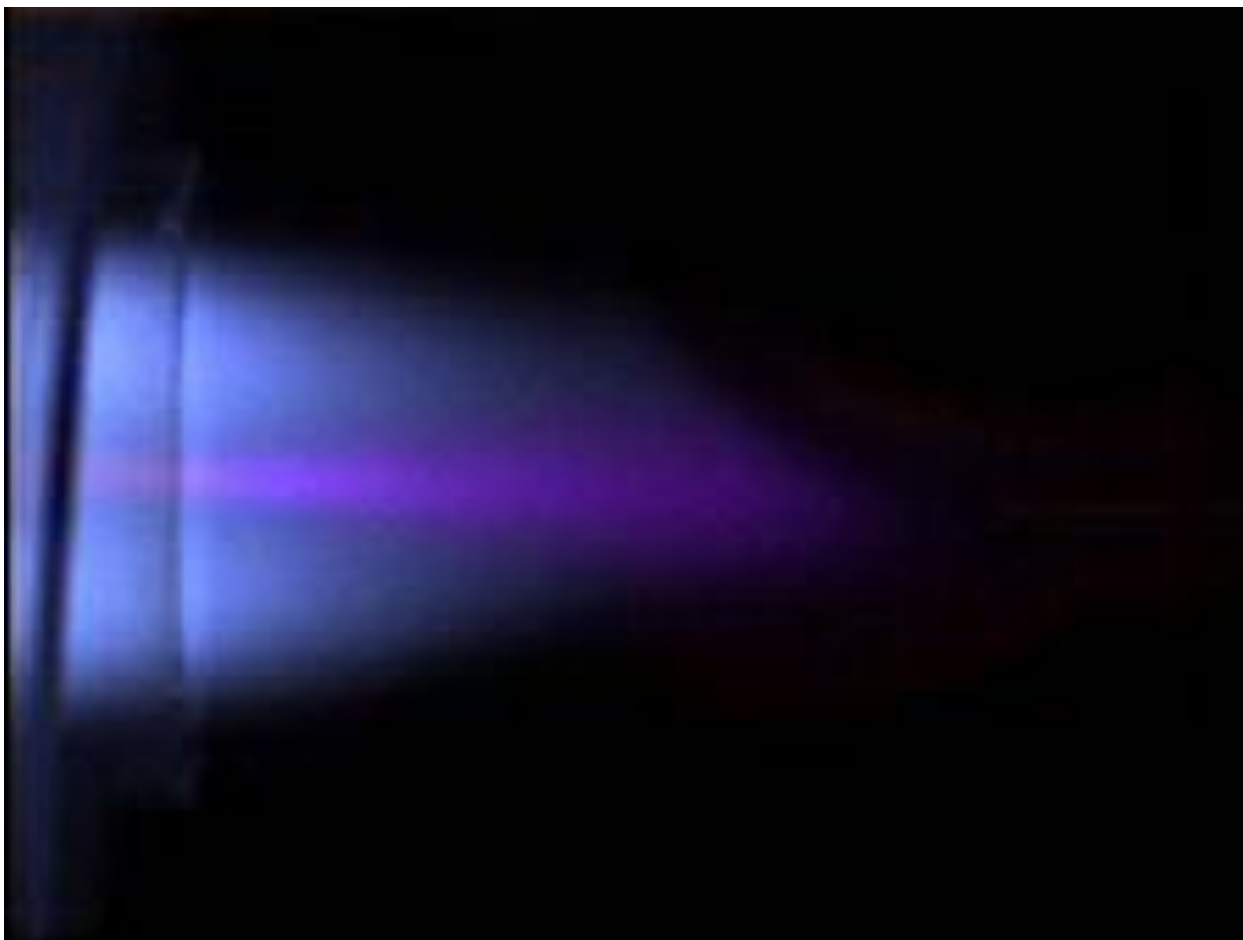
Figure 3. High speed photograph of the ICP during femtosecond laser ablation of NIST 610 glass in argon. This image is representative of the steady-state emission from fs LA when no discrete particle is traversing the plasma.
