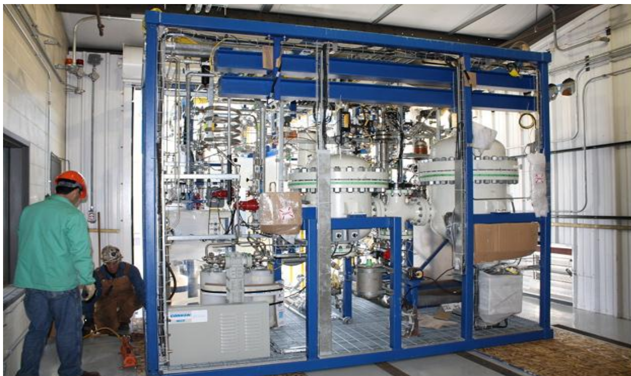
Figure 10-New IH 2 Continuous Pilot Plant being Positioned in GTI building
