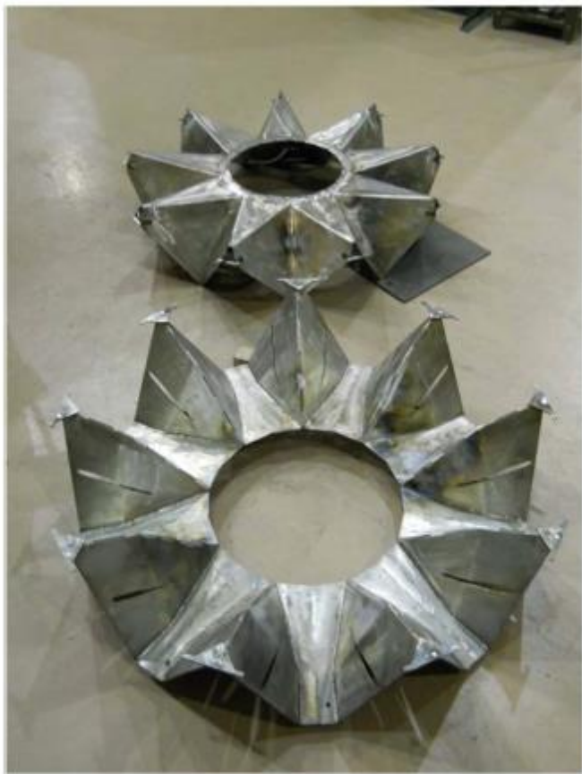
Figure 4. Photograph of the Saturn CSMITL anode (bottom) and cathode (top). The cathode is shown inverted from its operational condition to show the MITL surfaces and the pattern of metal erosion from electron loss along the ridgeline line of the tents.
