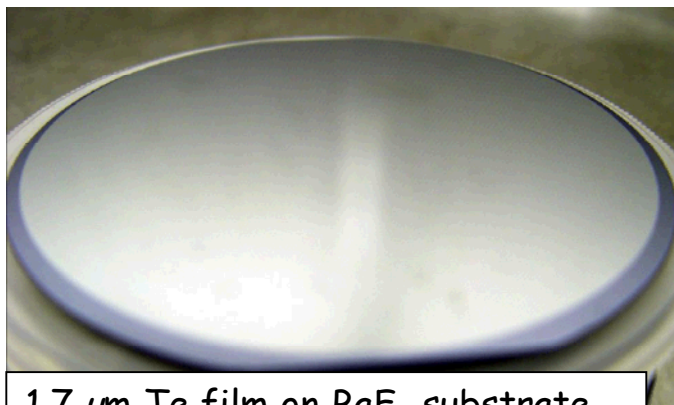
1.7\ \mu\text{m} Te film on \text{BaF}_2 substrate
