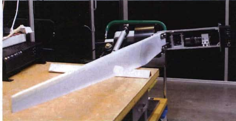
Figure 2: Photograph of LANL's Rotating PIV apparatus (Patent in progress). The diagnostic is designed to capture blade boundary layers under dynamic stall at any phase angle of rotation. This apparatus is also capable of non-intrusively measuring local blade inflow conditions.
