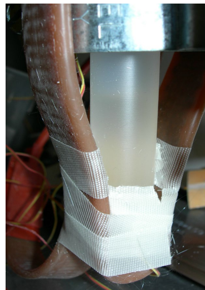
Figure 3. Auxiliary containment for \text{UF}_6 liquid studies at left; close-up of Kel-F container with liquid \text{UF}_6 at right.
