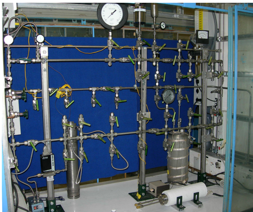
Figure 2. Test Loop configured for F 2 and heat treating a NaF chemical trap (the vertical cylinder in the lower left quadrant).
