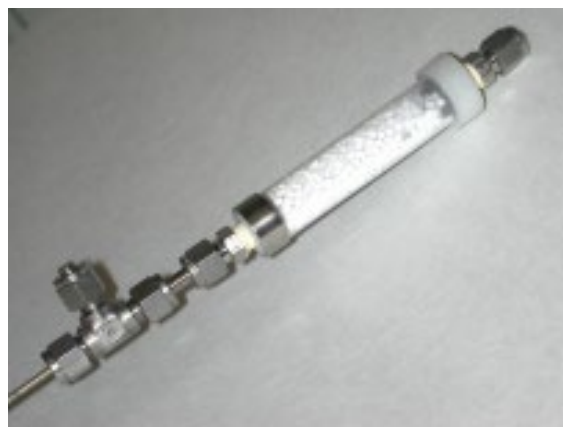
Figure 8. Miniature \text{NaF} -containing chemical trap used for determining loading behavior of \text{HF} on Morita \text{NaF} pellets.
