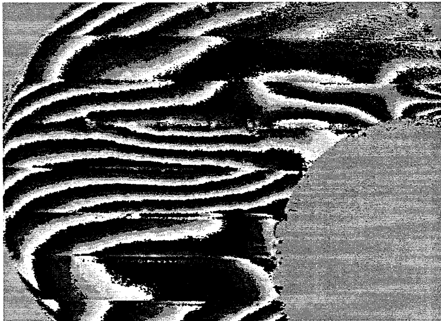
Figure 3: Typical wrapped fringe pattern \sigma_0 = 0.86 MPa.
