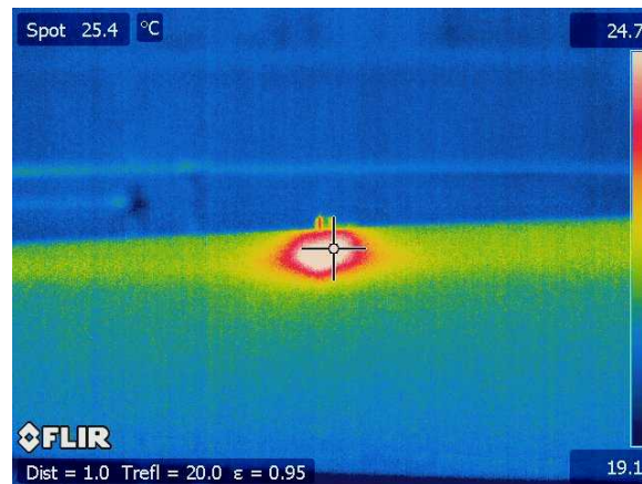
Figure 13 – Thermal Image of Out-of-Plane Wave Defect under Fatigue Loading
