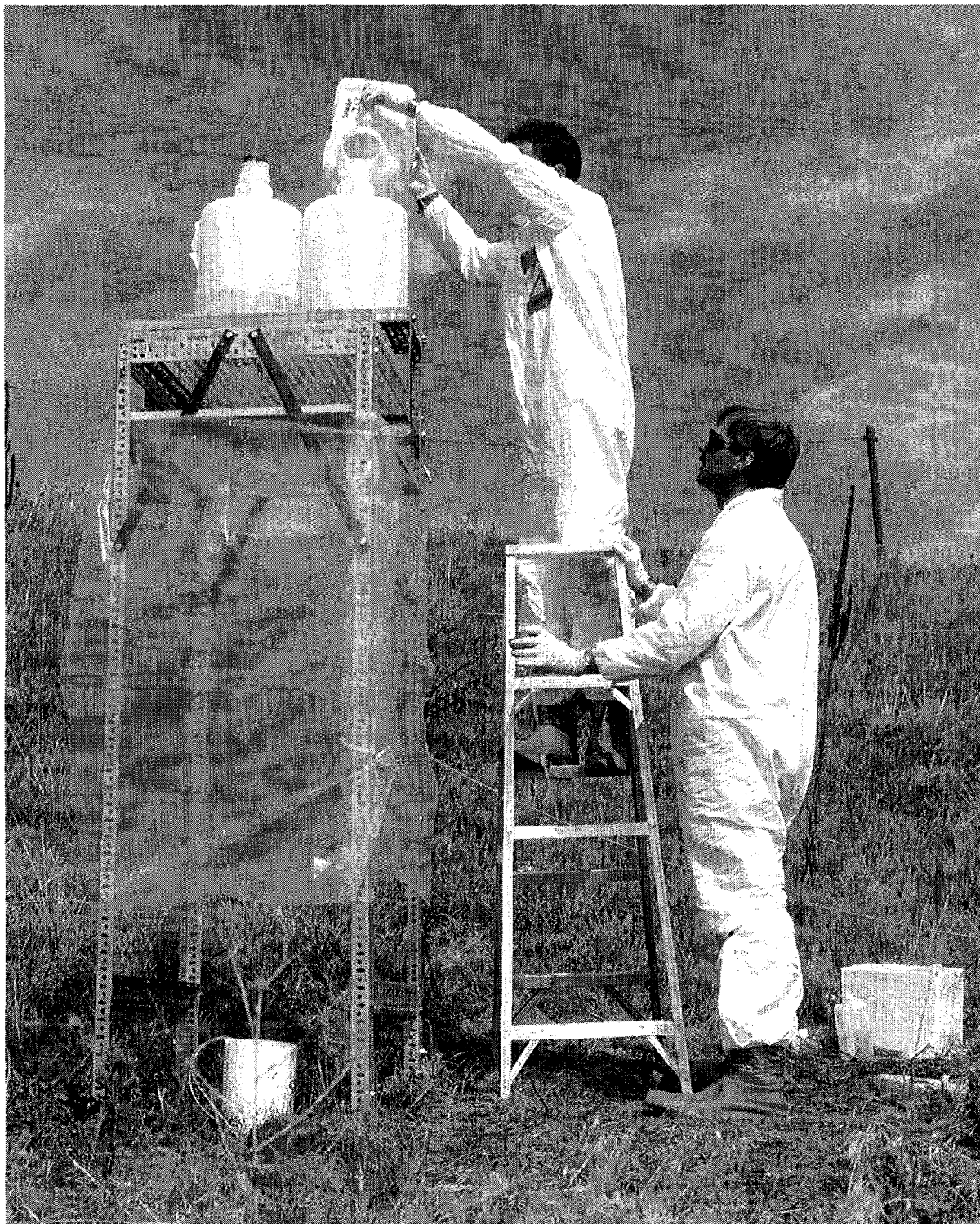
Figure 3. Conducting rainfall simulation experiments at Rocky Flats.
