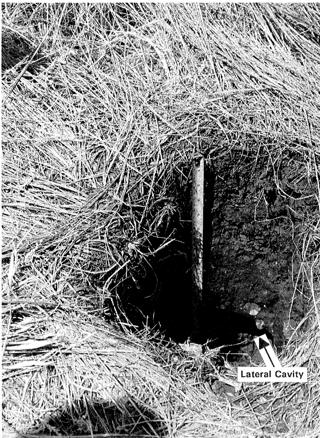
Figure 2. Manual installation of the ZTLs required digging a small access hole and placing the lysimeter under an undisturbed portion of the soil.
