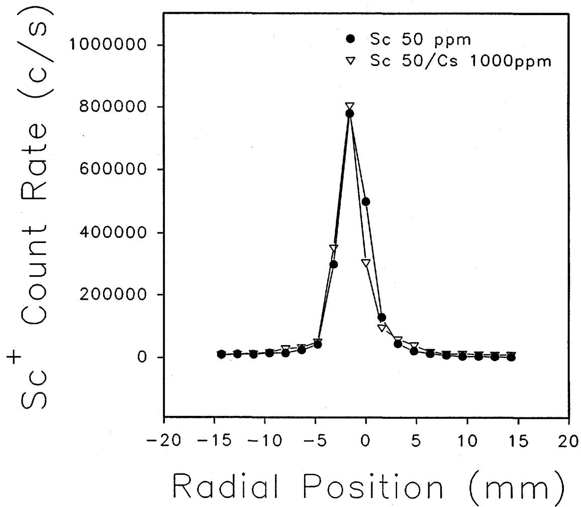
Figure 9. Effect of Cs matrix ( $1000 \text{ mg L}^{-1}$ ) on Sc beam profile, lens setting 2.
