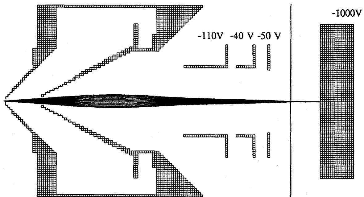
Figure 4. SIMION ion trajectories for ion lens setting 1.
