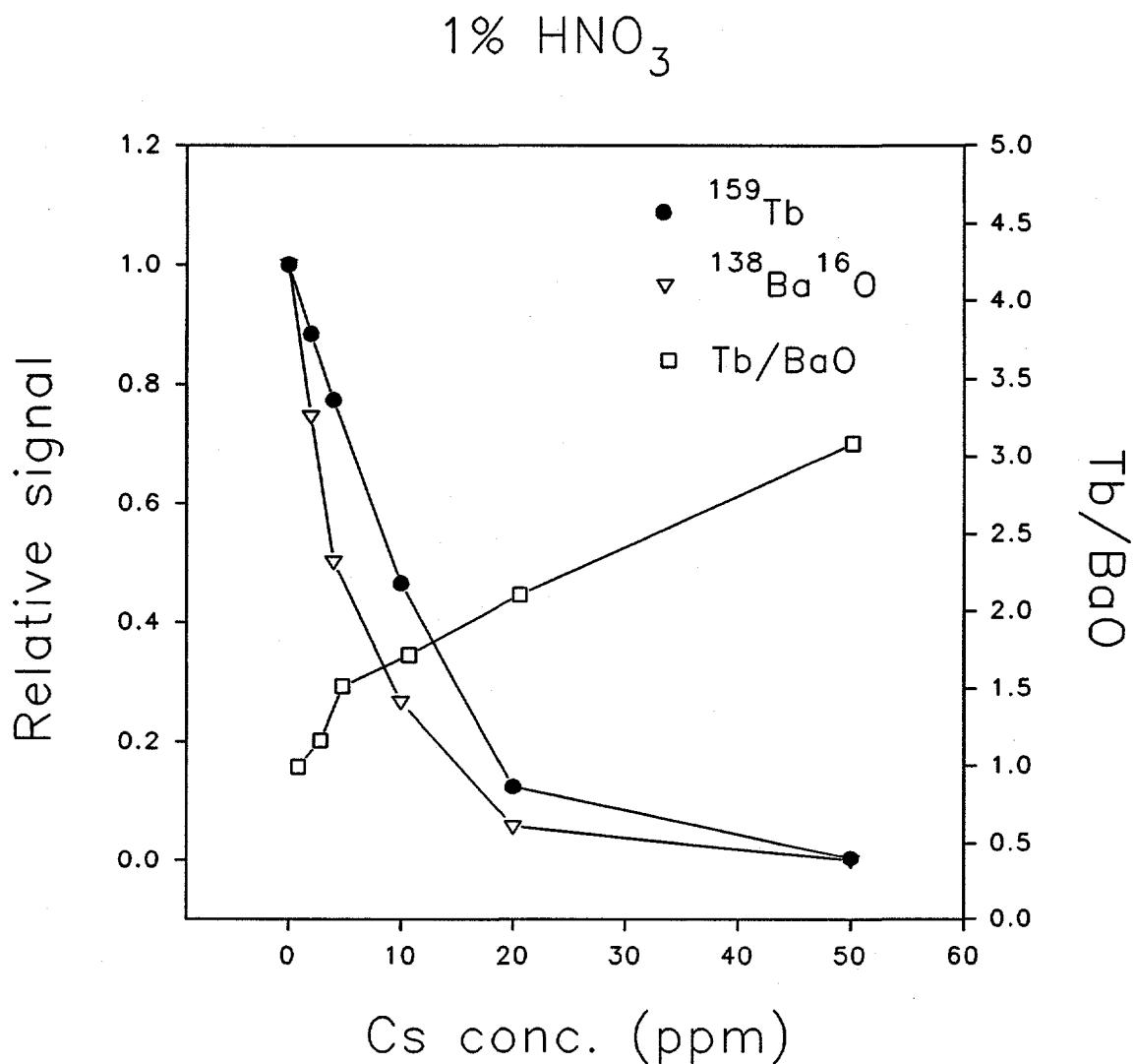
Figure 4.  $^{138}\text{Ba}^{16}\text{O}^+$  as internal standard for  $^{159}\text{Tb}^+$ .
