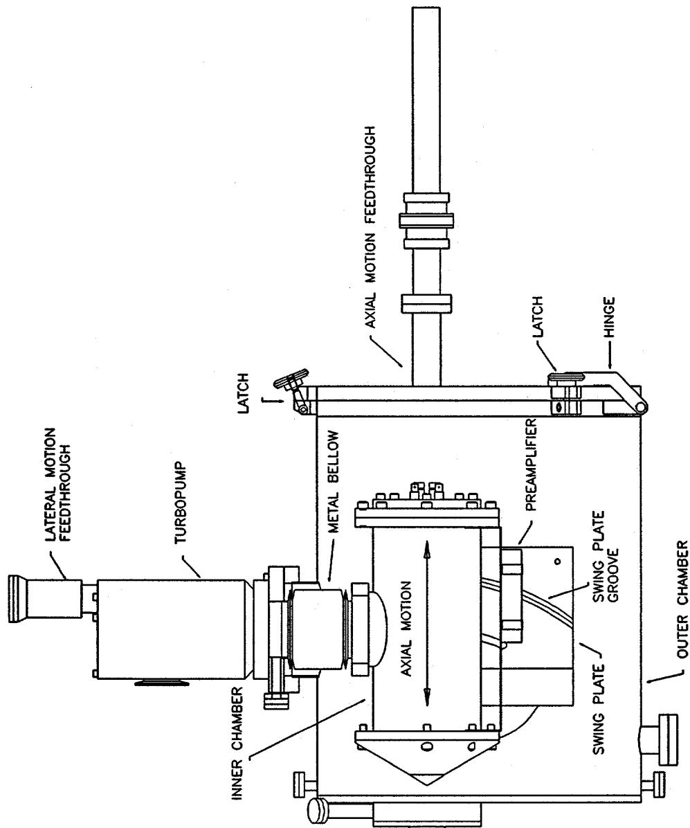
Figure 6. Top view showing axial motion of the inner chamber.
