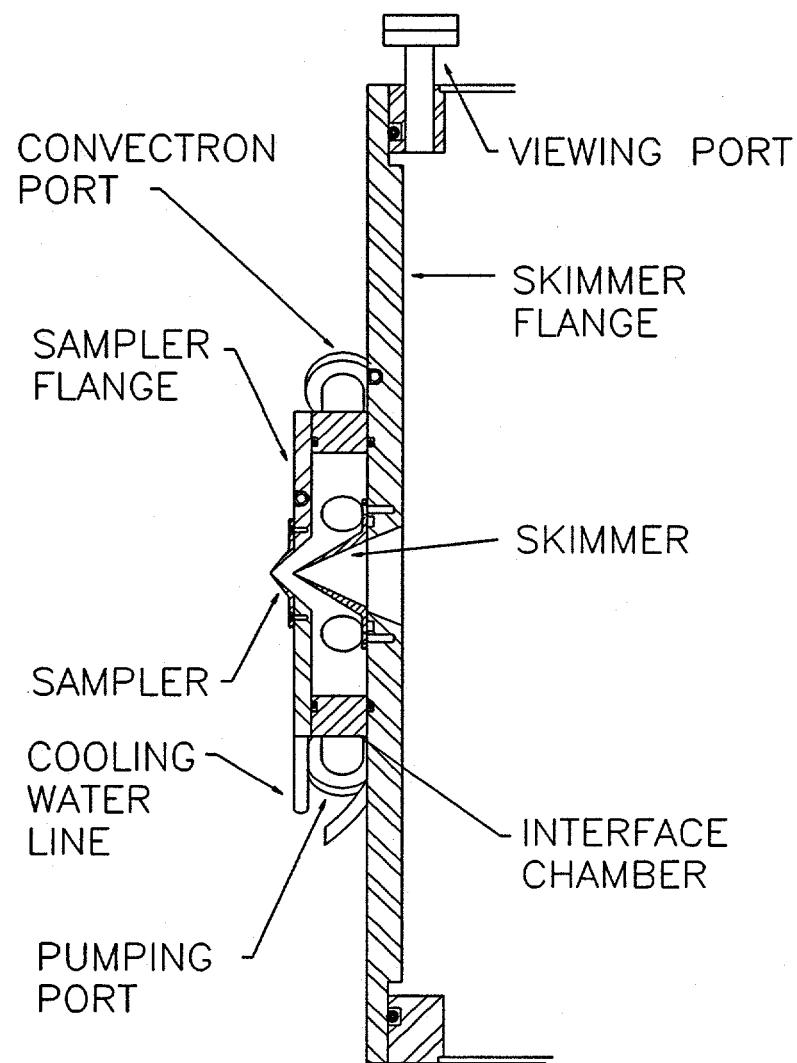
Figure 8. Section view of the ICP-MS interface.
