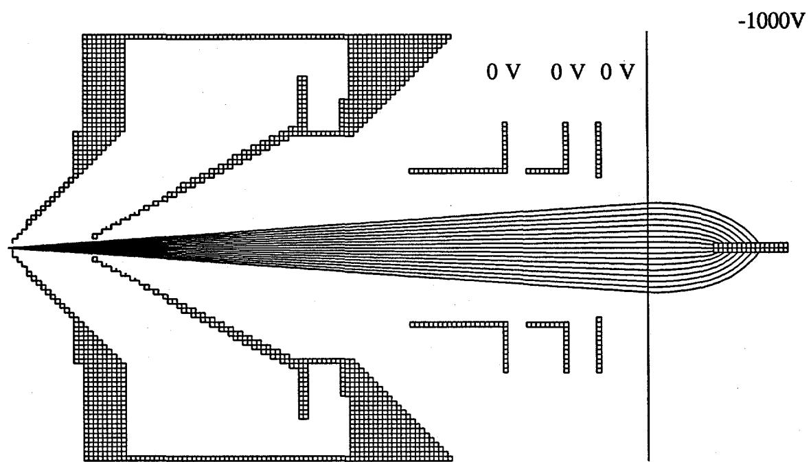
Figure 3. SIMION ion trajectory simulation with all the ion lenses set at ground potential. This is a side view of Figure 2, i.e., the Y-Z plane from Figure 1. The two grids at the right represent the thickness of one of the target electrodes.
