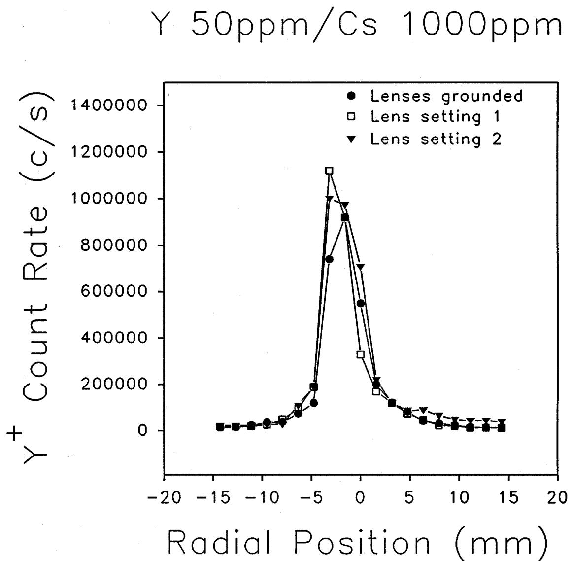
Figure 14. Effect of lens settings on Y beam profile, with Cs matrix at 1000 ppm.
