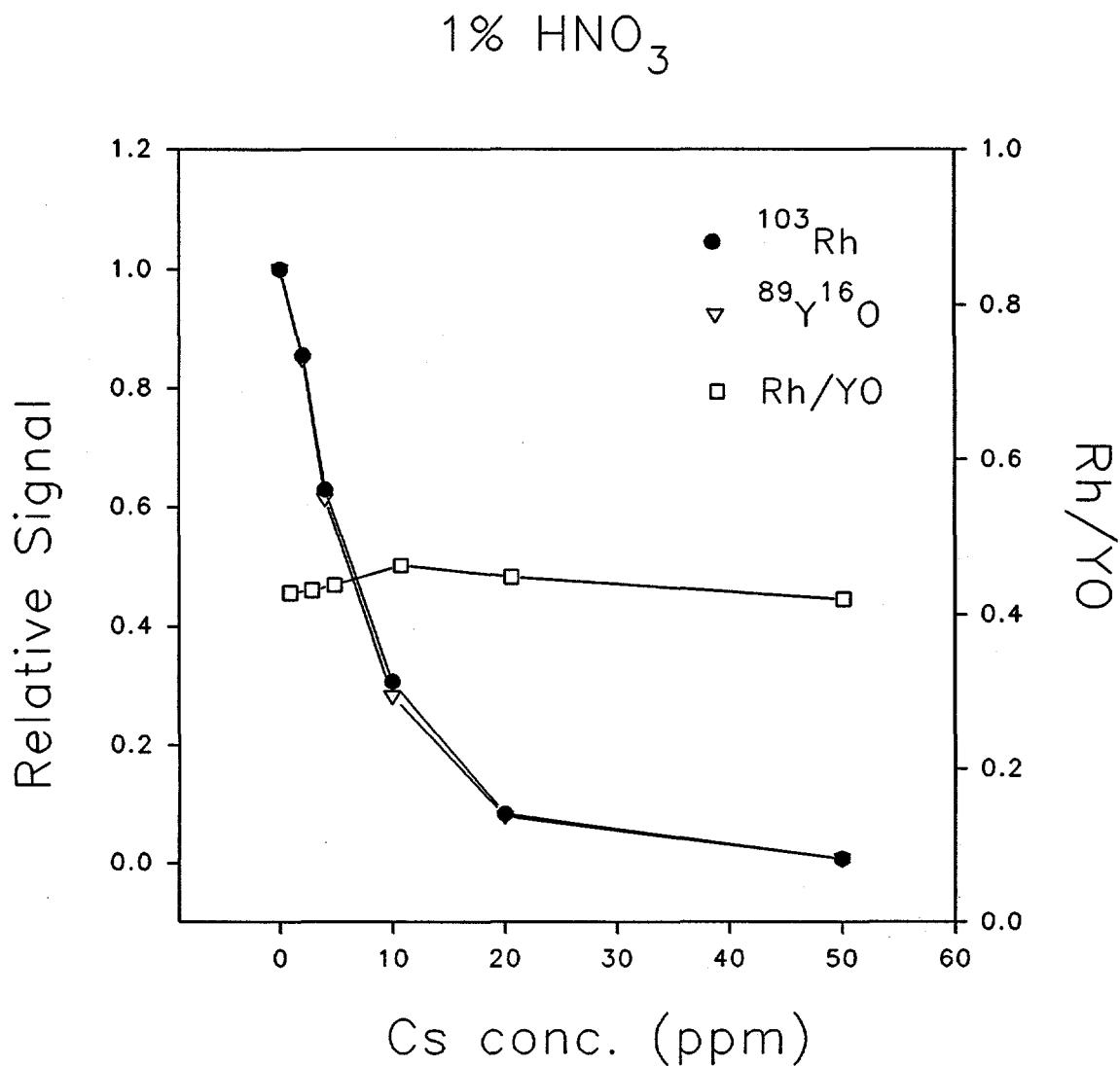
Figure 3.  $^{89}\text{Y}^{16}\text{O}^+$  as internal standard for  $^{103}\text{Rh}^+$ .
