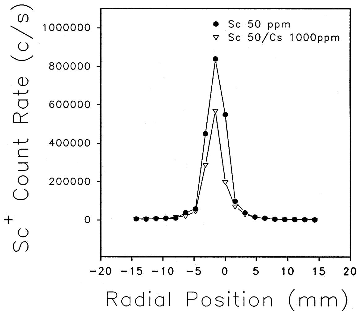
Figure 8. Effect of Cs matrix ( $1000 \text{ mg L}^{-1}$ ) on Sc beam profile, lens setting 1.
