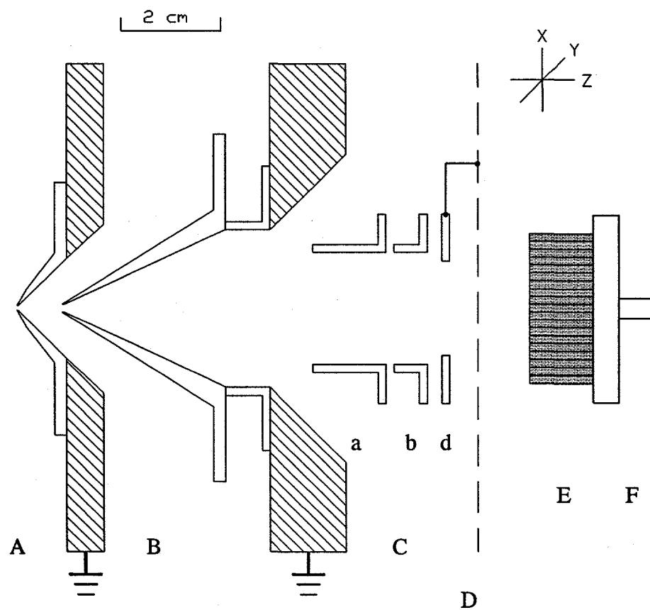
Figure 1. Top view of deposition apparatus. The targets were oriented horizontally. A: sampler. B: skimmer. C: ion optics, including the following elements: a: first cylindrical ion lens, b: second cylindrical ion lens, c: photon stop (not shown here, see Figure 6), d: plate ion lens. D: grid. E: graphite targets. F: water cooled mounting clamp and stand off, potential of -1000 V was provided by an electric feedthrough connected to a high voltage power supply.
