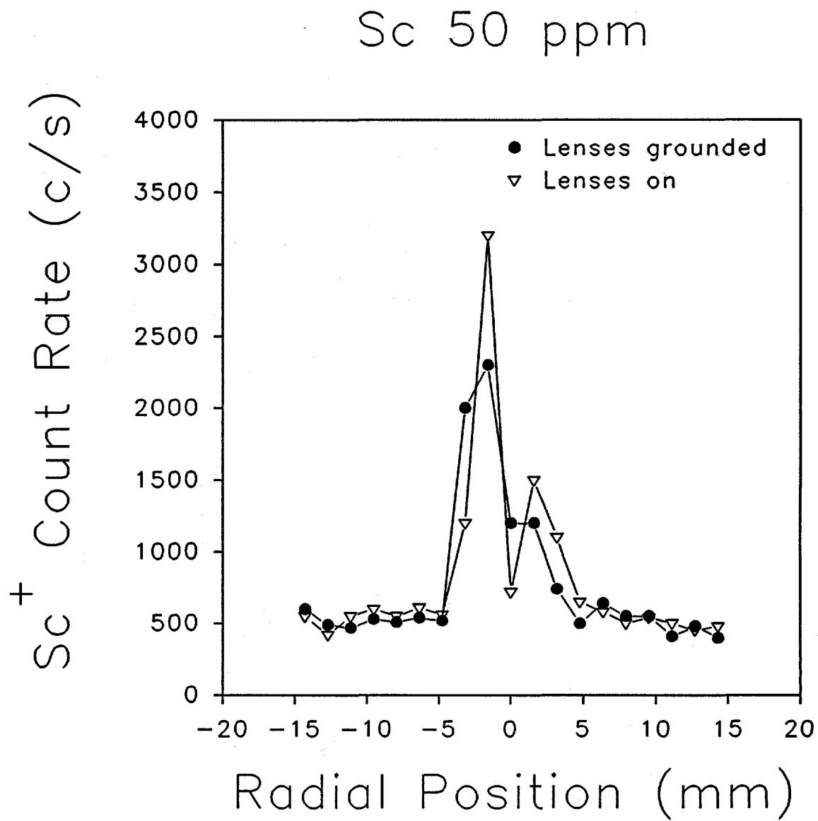
Figure 11. Beam profile for Sc at 50 mg L<sup>-1</sup> with a photon stop. There is less of a dip in the center with the lenses grounded.
