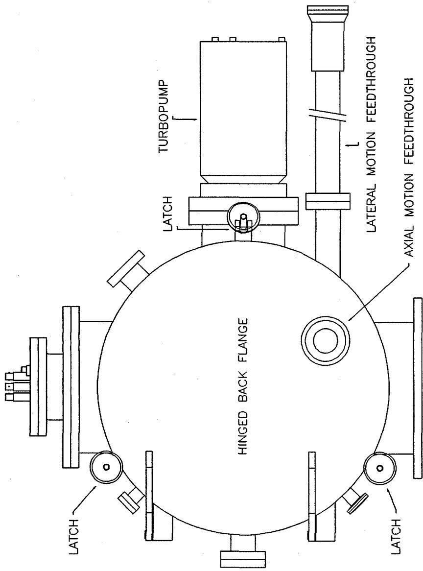
Figure 10. Rear view of the ICP-MS device.
