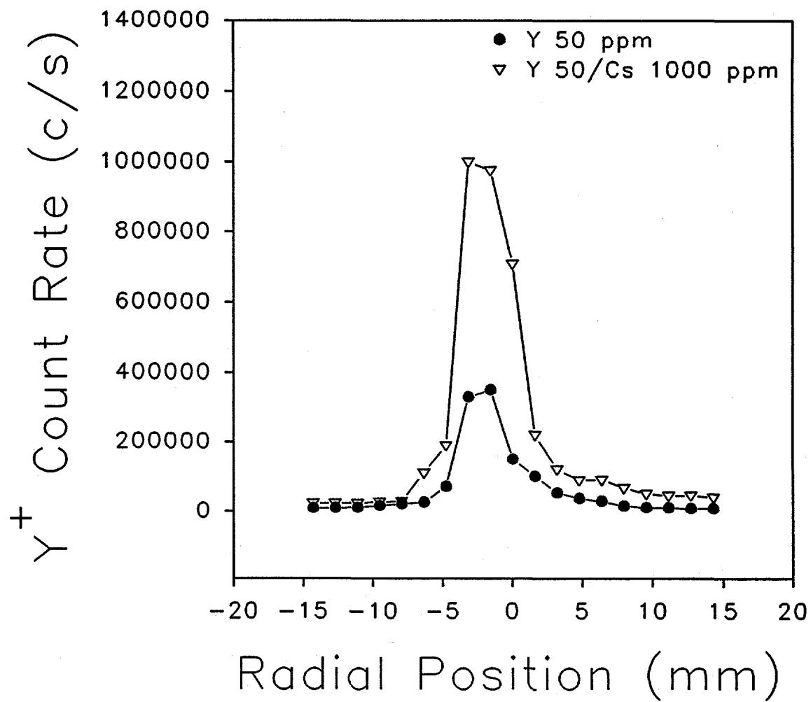
Figure 16. Effect of Cs matrix ( $1000 \text{ mg L}^{-1}$ ) on Sc beam profile, lens setting 2.
