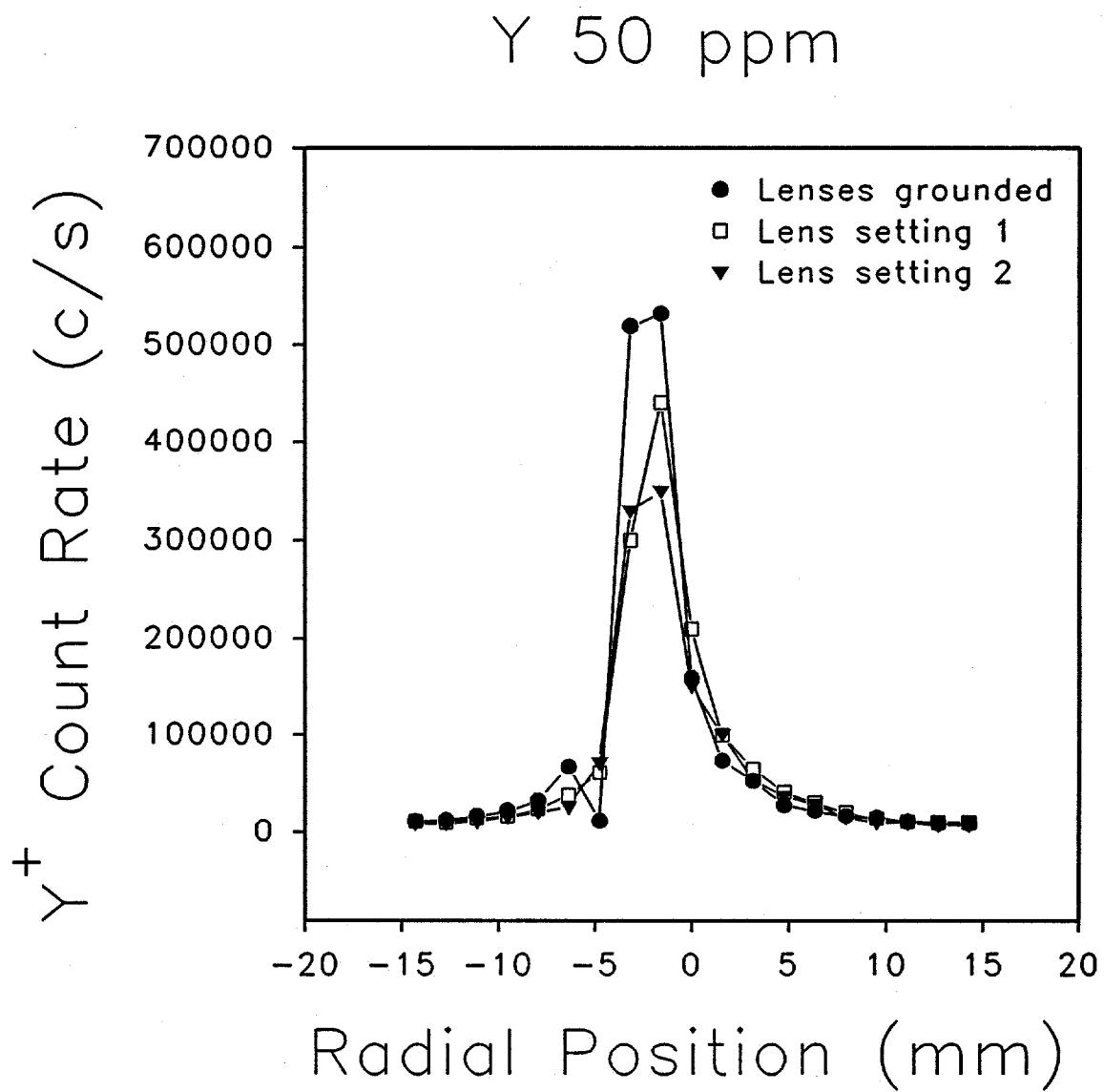
Figure 13. Effect of lens settings on Y beam profile.
