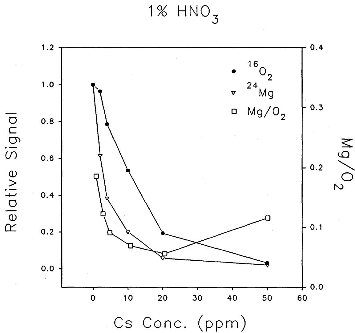
Figure 2.  $^{16}\text{O}_2^+$  as internal standard for  $^{24}\text{Mg}^+$ .
