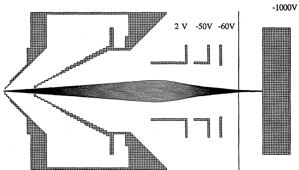
Figure 5. SIMION ion trajectories for ion lens setting 2.
