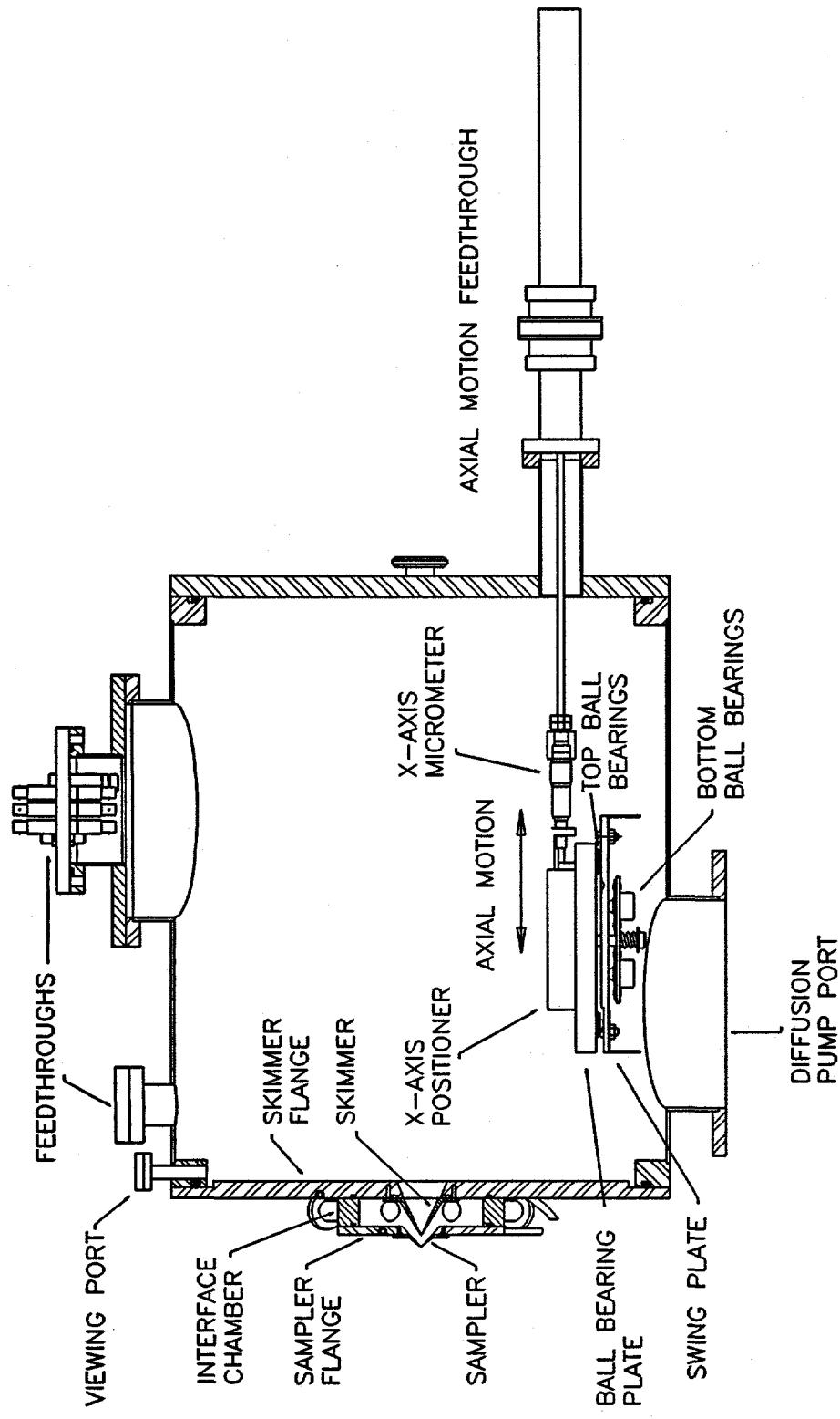
Figure 5. Section view of the ICP-MS device. Axial motion is provided by the axial motion feedthrough.
