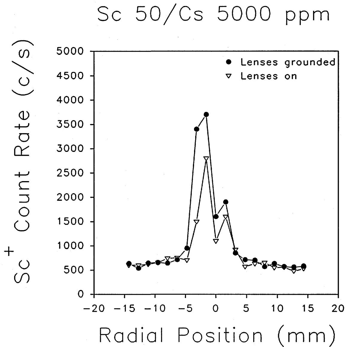
Figure 12. Beam profile for Sc at 50 mg L<sup>-1</sup> with Cs matrix at 5000 mg L<sup>-1</sup> and a photon stop. With matrix element present, grounding the lenses gives moderately higher signals than biasing them.
