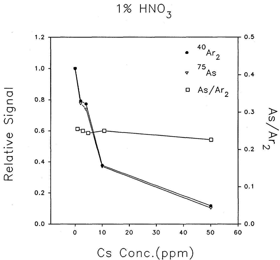
Figure 1.  $^{40}\text{Ar}_2^+$  as internal standard for  $^{75}\text{As}^+$ .
