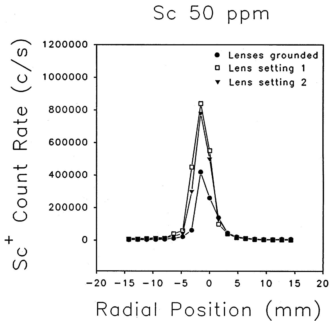
Figure 7. Deposition profile for Sc at 50 mg L<sup>-1</sup>.
