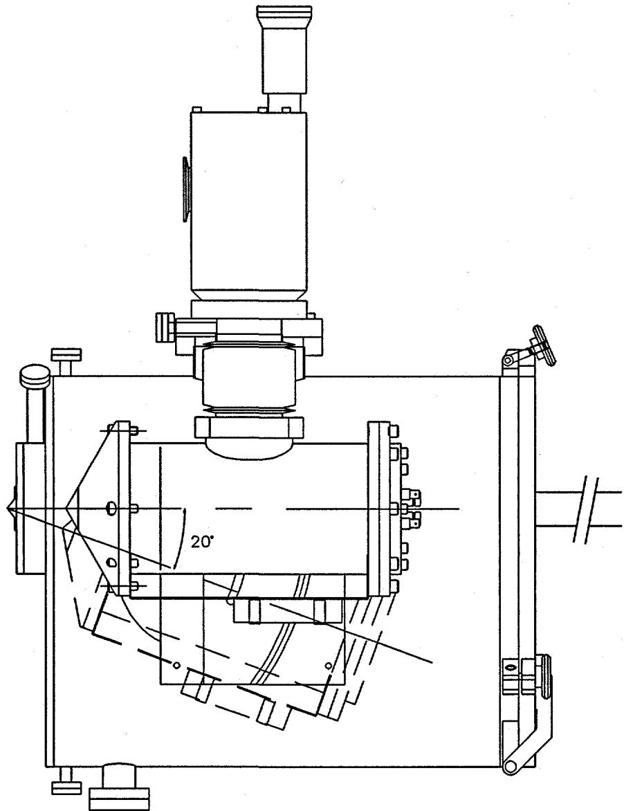
Figure 4. Lateral motion of the inner chamber. The maximum pivoting angle is 20°.
