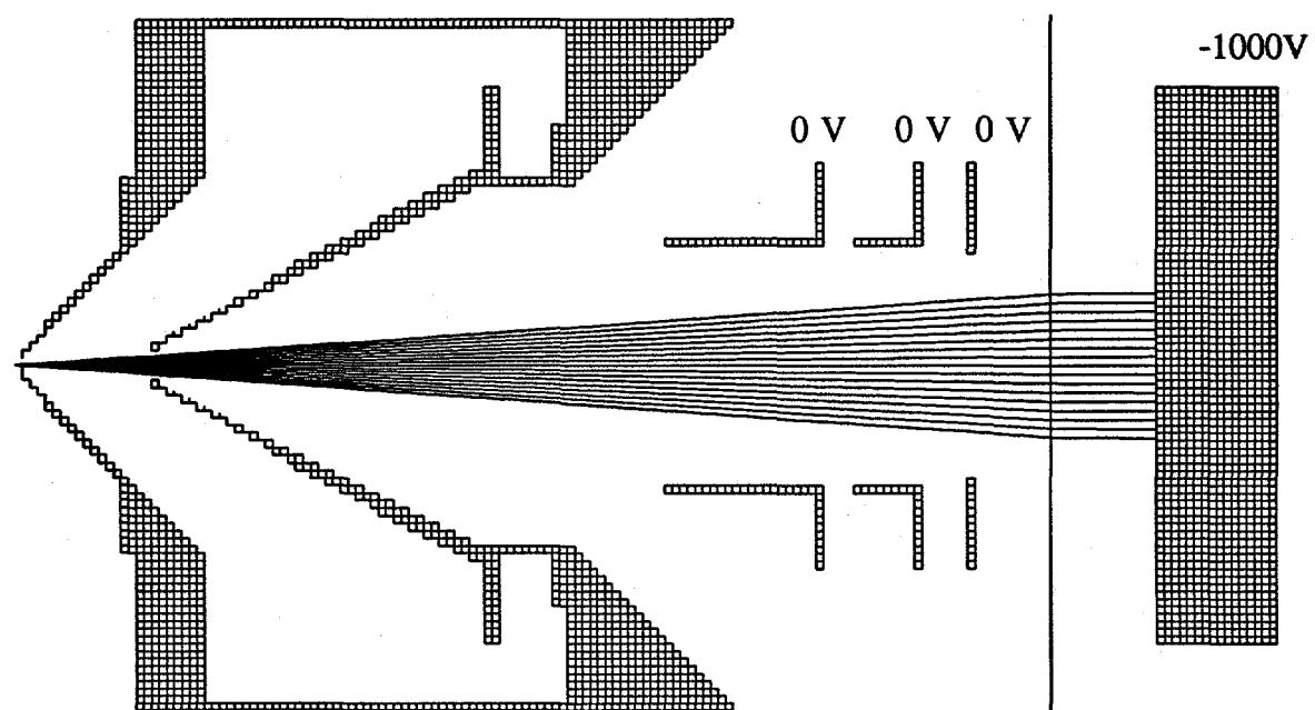
Figure 2. Top view of the SIMION ion trajectory simulation with all the ion lenses set at ground potential. This is the X-Z plane shown in Figure 1. The grids at the right represent the deposition targets. Each grid is 0.94 mm wide in this and Figs. 3-6.
