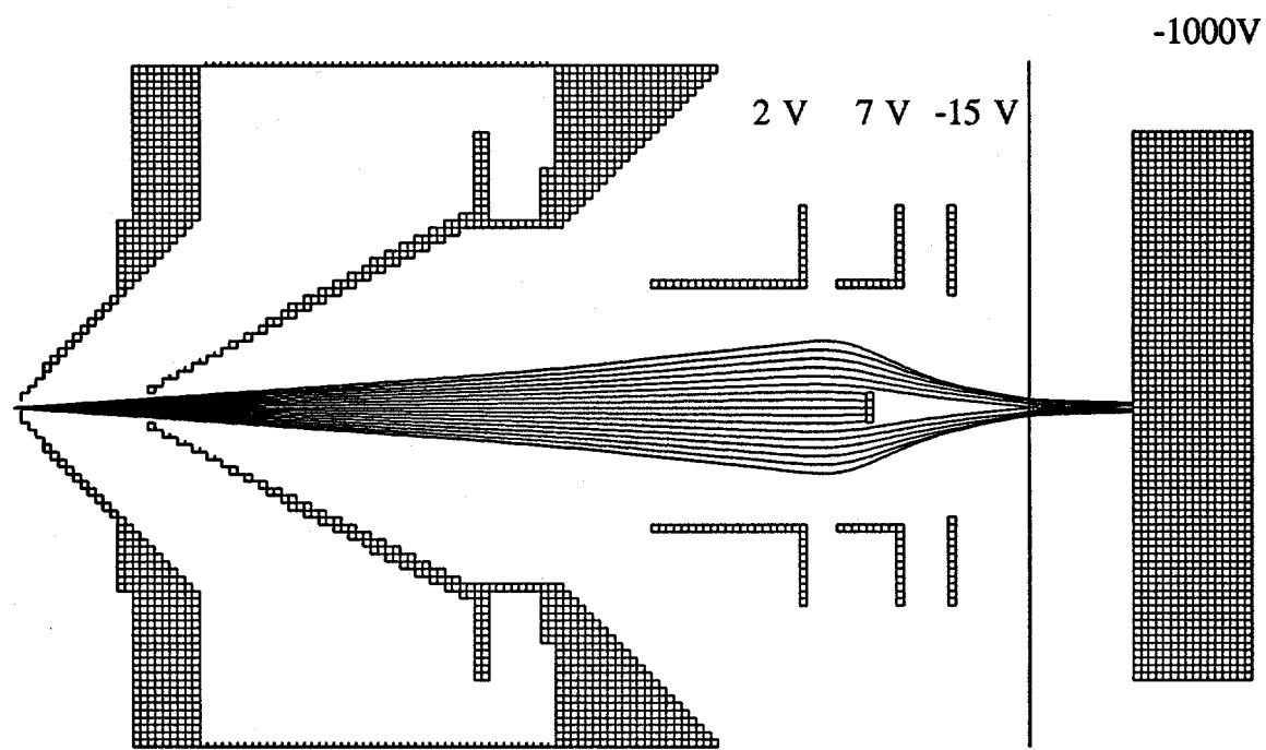
Figure 6. SIMION ion trajectories for ion lens setting 3 where a photon stop is present.
