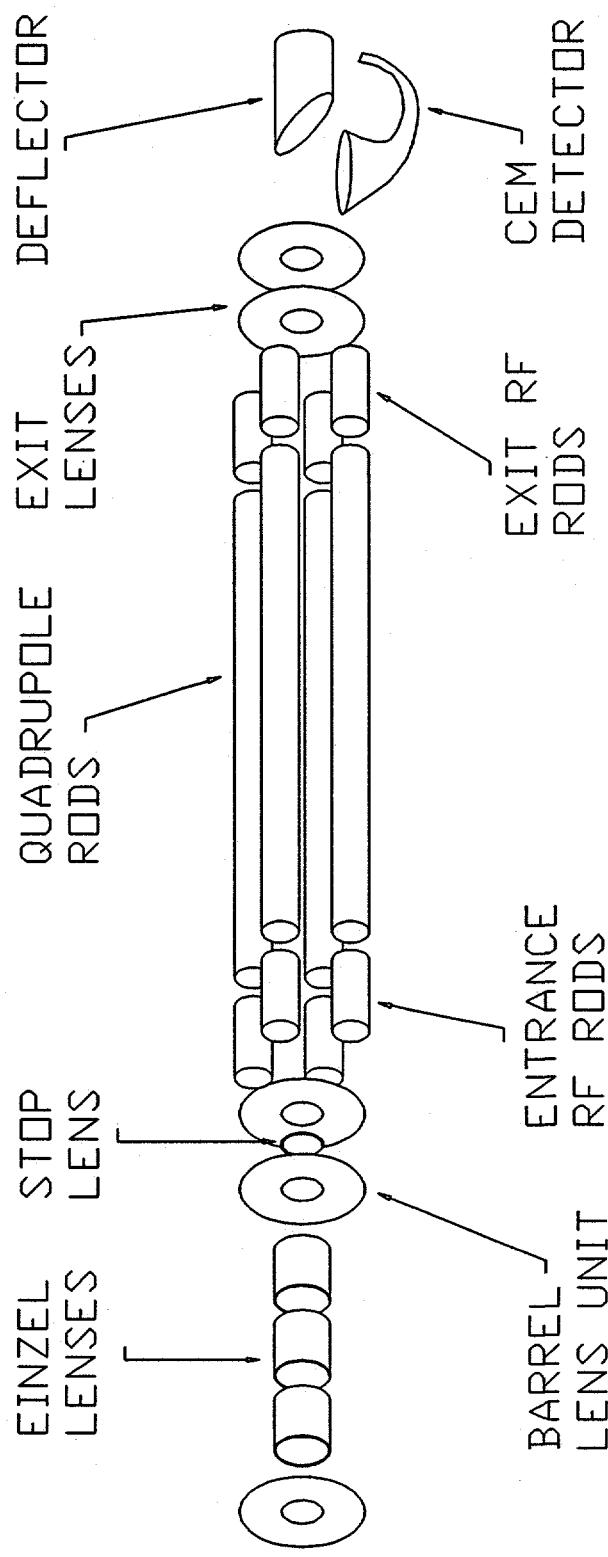
Figure 2. Illustration of a mass spectrometer in ICP-MS.
