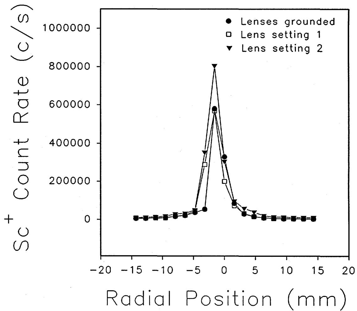
Figure 10. Effect of lens settings on Sc beam profile, with Cs matrix at  $1000 \text{ mg L}^{-1}$ .
