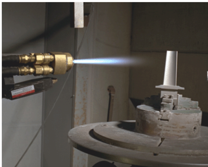
Figure 3-3. Plasma thermal spray coating. (NASA)
