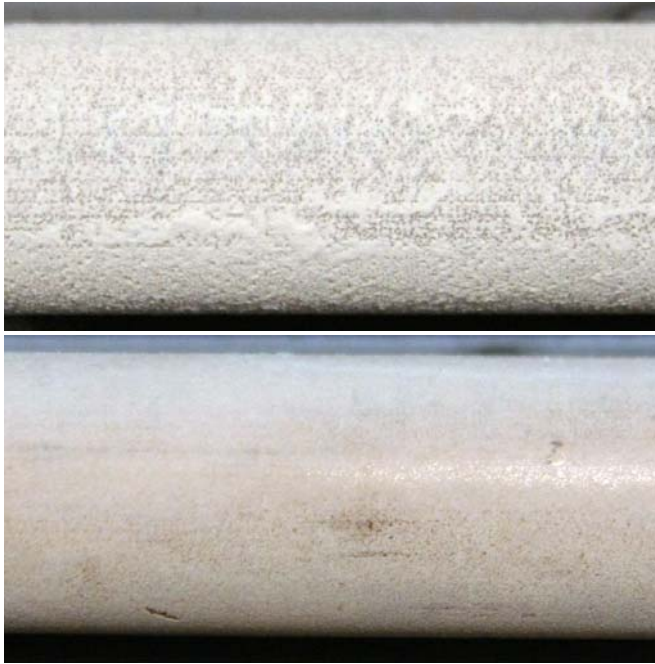
Figure 6-28. Photographic images of the scales for (a) no-treatment; (b) plasma treatment cases ( \text{CaCO}_3 hardness of 250 ppm and a flow velocity of 0.1 m/s) (Yang et al., 2010b).
