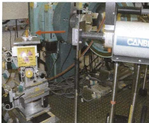
Figure 1. Picture of experimental setup showing the multi-stage assembly for positioning of the sample holder and the HPGe detector. The monochromatic synchrotron beam enters from the right, shown by the arrow inset.
