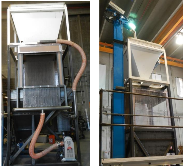
Figure 12. Assembled particle-receiver system. Left: particles being released through receiver. Right: side-view showing Lexan panels for viewing particles falling through the receiver.
