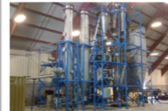
A gasifier being used by a NAABB partner to convert algal biomass to fuels
