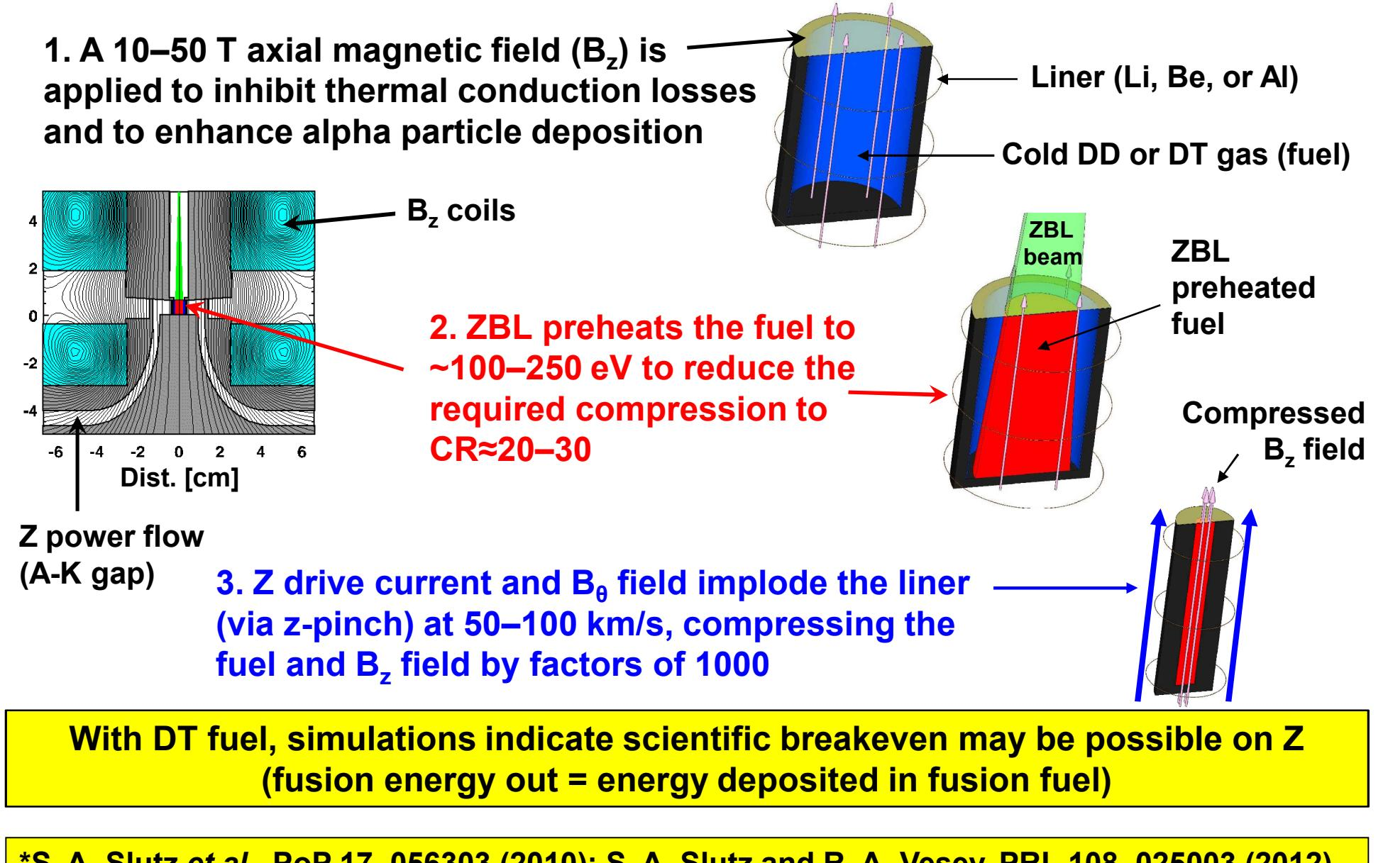
Our ability to compress flux remains unclear, however, due to poorly understood physics. For example, the Nernst thermo-electromagnetic effect can cause significant flux loss across strong temperature gradients in the fuel. The Nernst effect is included in higher-order magnetohydrodynamics theory, but the physics needs to be validated experimentally.
