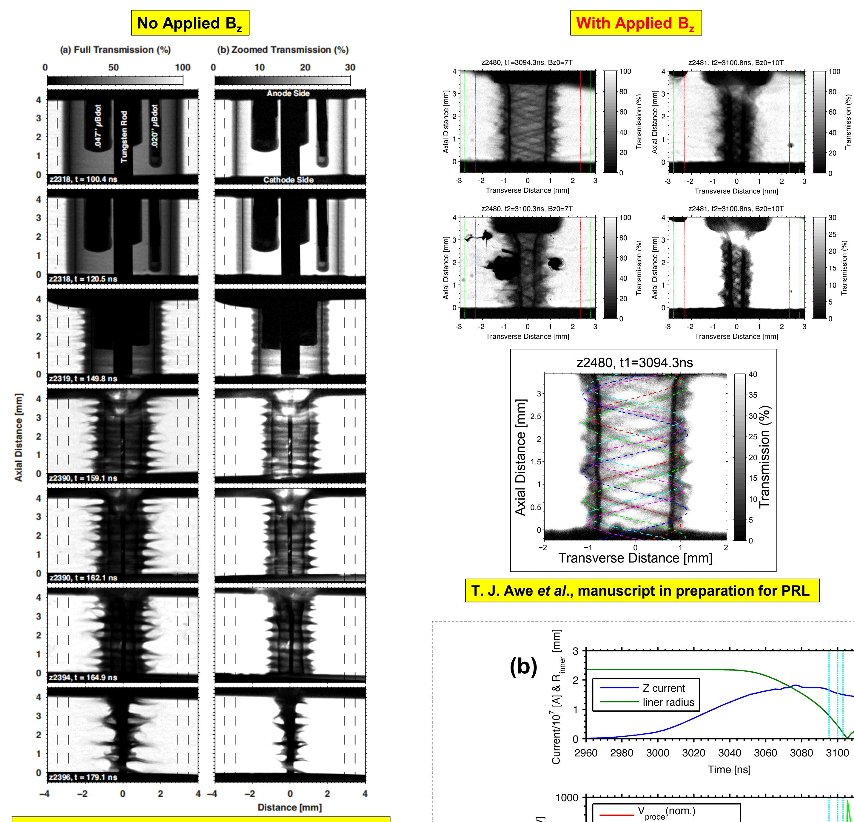
(a) We have developed simulation codes to calculate the magnetic fields during flux compression. (b) We have used these simulations to estimate the expected signal responses from μBdot probes in the fringe fields. (c) We have used these estimates to compare to our first attempts to experimentally measure the flux compression fringe fields with μBdot probes:
