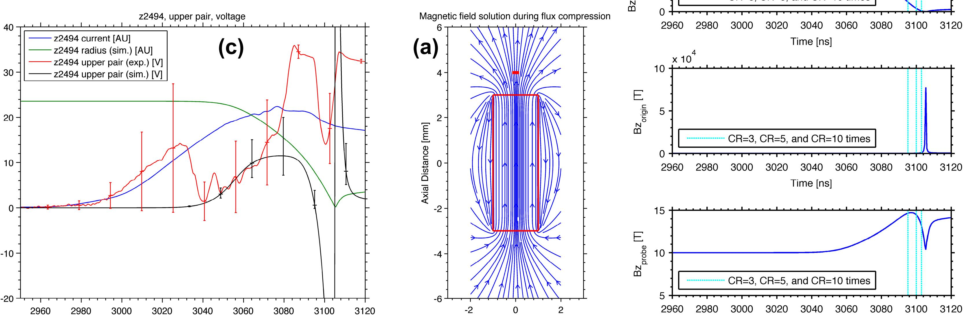
We have already successfully detected flux compression signals, but we have also learned that it will be very difficult to infer the amplified  $B_z$  field within the liner at CR=3, 5, or 10 (our measurement goals) without very precise characterization of the probe loop positions and better electrical shielding
