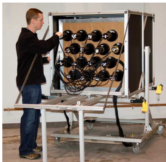
Figure 2. The neutron Scatter Camera deployed for neutron spectrum measurement.
