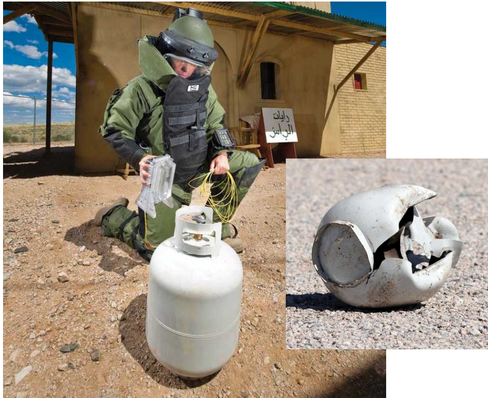
Stingray destroys propane tank with a blade of water
