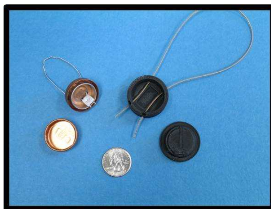
Figure 1: Size comparison of a metal cup seal (left), rapid prototype of an early model of the Ceramic Seal (right), and a U.S. quarter (bottom).
