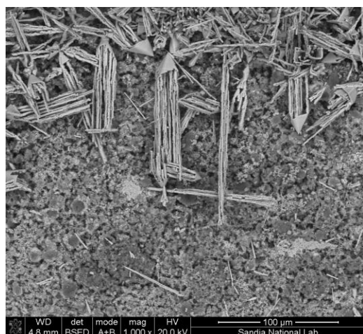
Fig. 7. SEM image of a 15 wt% AgI-MOR sample heated 550°C for 12 min after 7 days in water at 90°C.
