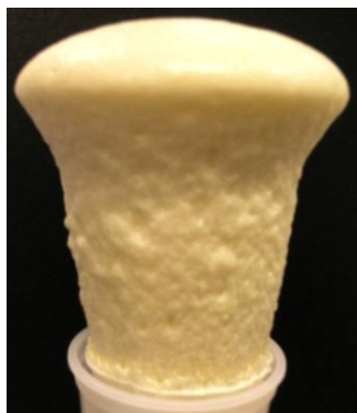
Figure 1. PMDI has a short pot-life: models can help reduce defects and improve filling process.
