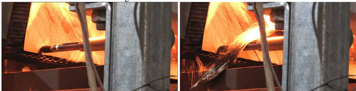
Figure 4. Photographs of the Test 43 ABDR panel in torsion before (left) and after (right) the first significant movement of the fibers.
