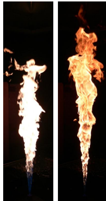
Fig. 2. Color digital SLR camera photographs of the ethylene jet flame (left) and the JP-8 surrogate jet flame (right).
