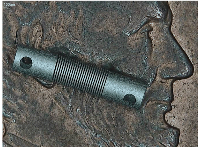
Fig. 1: Prototype meso scale extension spring on a penny.
