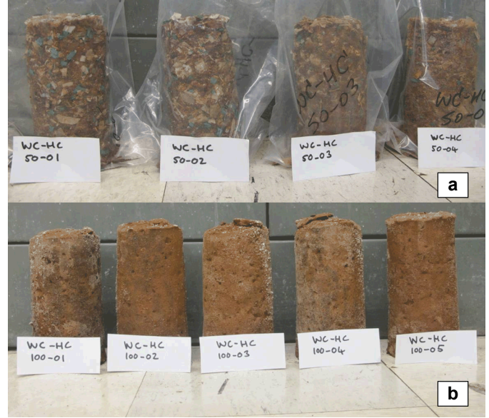
Fig. 14. Posttest 50% (a) and 100% (b) degraded hydrostatic compression samples.
