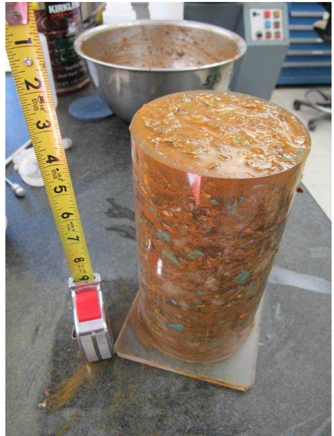
Fig. 2. Saturated 50% recipe contained within the ‘volume standard’ ready for insertion into gum rubber jacket assembly.
