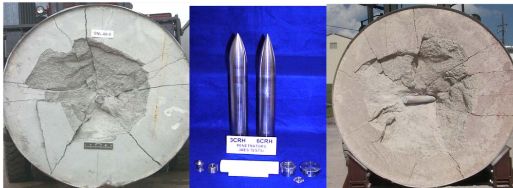
Normal & Oblique Impact Testing with Instrumented Penetrators
