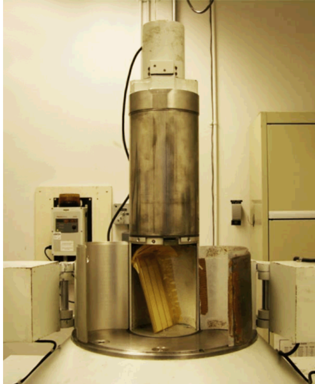
Figure 2. Photograph of test samples in the gamma cell.
