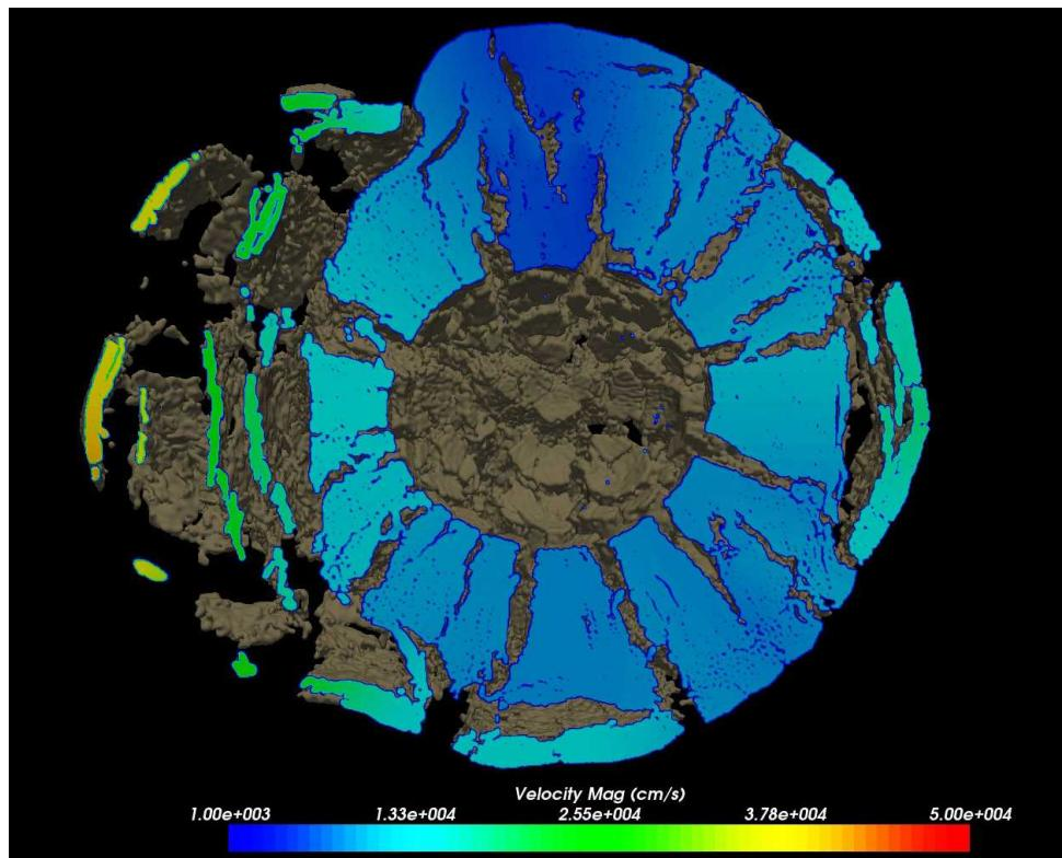
Asteroid Golevka measures about 500 x 600 x 700 meters. In this CTH shock physics simulation, a 10 Megaton explosion was initiated at the center of mass. The simulation ran for about 15 hours on 7200 nodes of Red Storm and provided approximately 0.65 second of simulated time.
