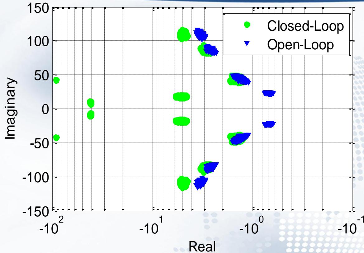
**The loci of eigenvalues for the open-loop and closed-loop systems of randomly generated plants**
