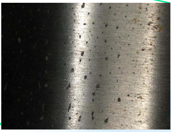
Directionality of pits near weld
