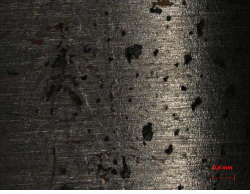
Directionality of pits near weld
