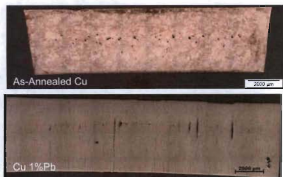
Figure 5. Optical images showing damage in high purity Cu and Cu-Pb after an incipient spall experiment. The top image corresponds to pure Cu whereas the bottom image is for Cu-Pb.
