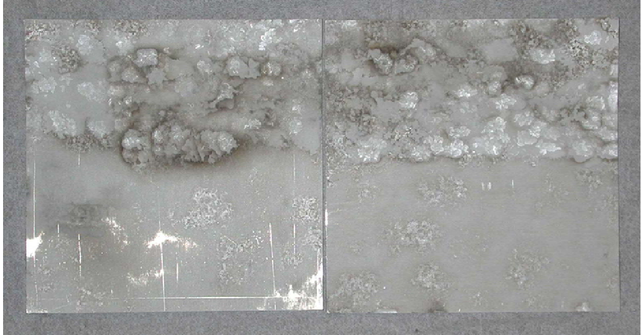
Figure 4.5. Sandwich 2.4a1. The top half of each square was TA cleaned and the bottom half continued arcing until roughened. This was not HIP'd due to EB weld failure during handling after welding.
