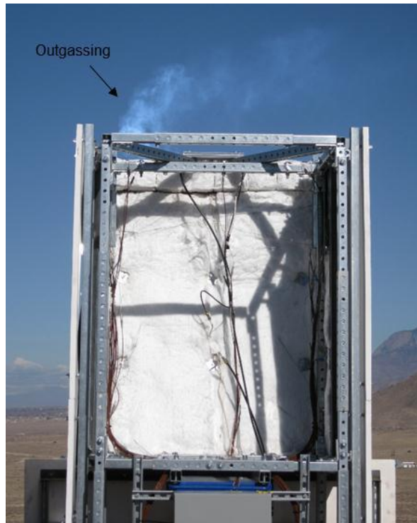
Outgassing During test
