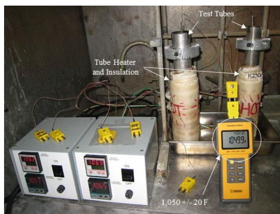
Molten Salt Exposure within Tubes
